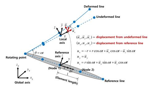
Fig. 1 Conceptual figure of FEM model of elastic rotating beam for blade
