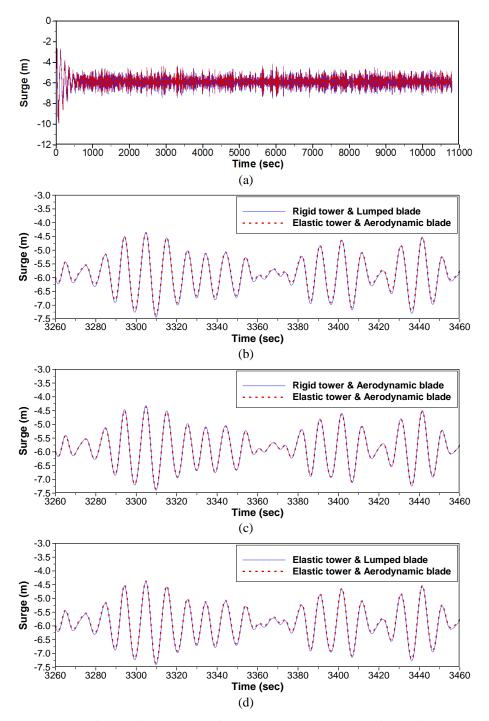
Fig. 3 (a) Comparison of surge in sea state 5 (full range), (b) Comparison of surge in sea state 5 (zoom range : case 1 vs 4), (c) Comparison of surge in sea state 5 (zoom range : case 2 vs 4) and (d) Comparison of surge in sea state 5 (zoom range : case 3 vs 4)
