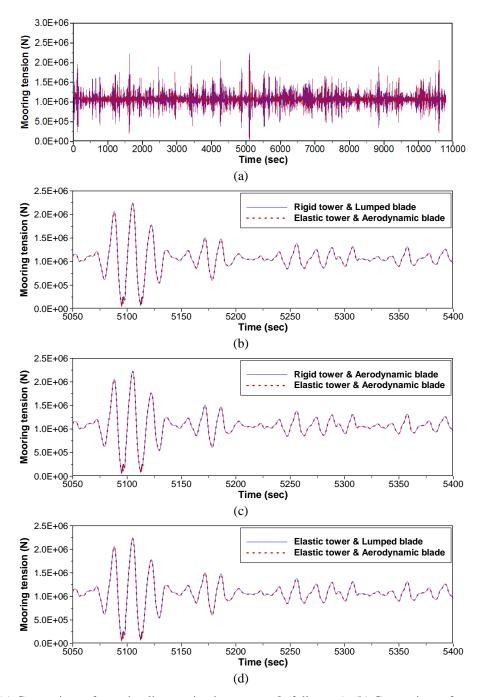
Fig. 11 (a) Comparison of mooring line tension in sea state 8 (full range), (b) Comparison of mooring line tension in sea state 8 (zoom range : case 1 vs 4), (c) Comparison of mooring line tension in sea state 8 (zoom range : case 2 vs 4) and (d) Comparison of mooring line tension in sea state 8 (zoom range : case 3 vs 4)
