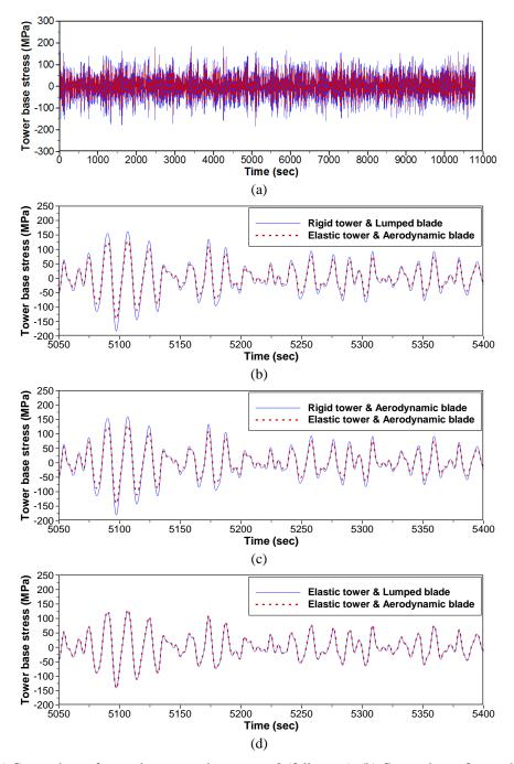
Fig. 12 (a) Comparison of tower base stress in sea state 8 (full range), (b) Comparison of tower base stress in sea state 8 (zoom range : case 1 vs 4), (c) Comparison of tower base stress in sea state 8 (zoom range : case 2 vs 4) and (d) Comparison of tower base stress in sea state 8 (zoom range : case 3 vs 4)
