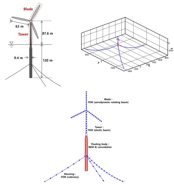
Fig. 2 Geometry of example wind turbine and its numerical model
