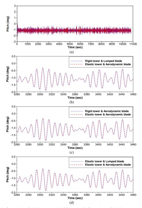
Fig. 5 (a) Comparison of pitch in sea state 5 (full range), (b) Comparison of pitch in sea state 5 (zoom range : case 1 vs 4), (c) Comparison of pitch in sea state 5 (zoom range : case 2 vs 4) and (d) Comparison of pitch in sea state 5 (zoom range : case 3 vs 4)
