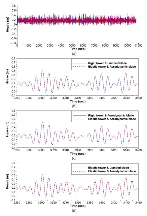
Fig. 4 (a) Comparison of heave in sea state 5 (full range), (b) Comparison of heave in sea state 5 (zoom range : case 1 vs 4), (c) Comparison of heave in sea state 5 (zoom range : case 2 vs 4) and (d) Comparison of heave in sea state 5 (zoom range : case 3 vs 4)
