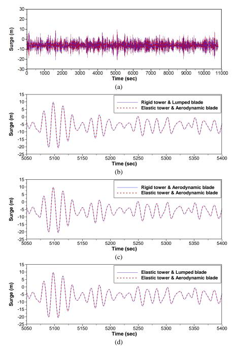
Fig. 8 (a) Comparison of surge in sea state 8 (full range), (b) Comparison of surge in sea state 8 (zoom range : case 1 vs 4), (c) Comparison of surge in sea state 8 (zoom range : case 2 vs 4), (d) Comparison of surge in sea state 8 (zoom range : case 3 vs 4)
