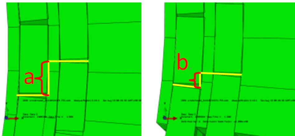
Fig. 7 Slipping of the tendon armors under load case 2
