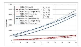
Fig. 8 Effects of  $\gamma$  on main diagonal terms of the LJF matrix for a symmetric K-joint
