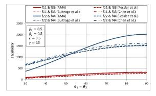
Fig. 7 Effects of  $\theta$  on main diagonal terms of the LJF matrix for a symmetric K-joint
