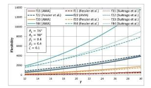
Fig. 14 Effects of  $\gamma$  on main diagonal terms of the LJF matrix for a Y-T joint
