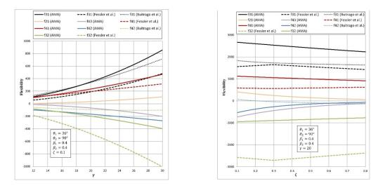
Fig. 24 Effects of  $\gamma$  on non-diagonal terms of the Fig. 25 Effects of  $\zeta$  on non-diagonal terms of LJF matrix for a Y-T joint the LJF matrix for a Y-T joint
