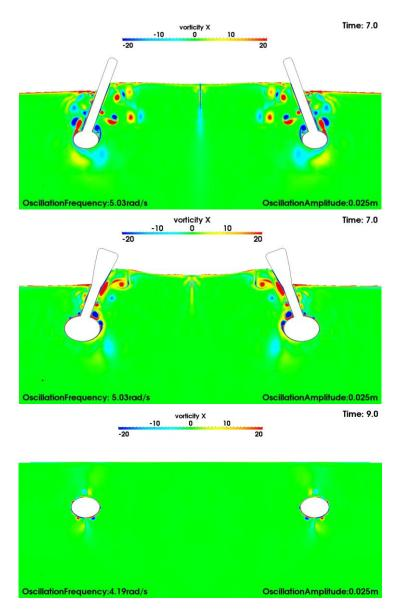
Fig. 4 Snapshot of the predicted viscous flow field (vorticity) for station 1, 4 and 6 respectively for the heave radiation problem
