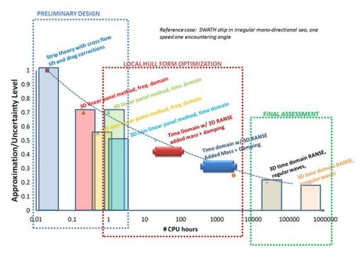
Fig. 2 Accuracy vs. computational time of different numerical methods for the motion prediction of SWATH ship in waves. Considered methods range from 2D potential flow theories to unsteady 3D viscous flow solvers
