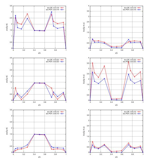
Fig. 5 Sectional heave added mass (a<sub>33</sub>) and damping (b<sub>33</sub>) calculated with inviscid (POT) and viscous (OF) methods at three different oscillation frequencies plot along ship length
