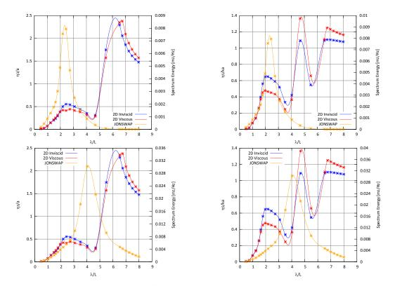
Fig. 7 Response Amplitude Operators of Heave ( $\eta_3$ ) and Pitch ( $\eta_5$ ) calculated by the two methods with JONSWAP
