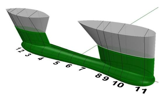
Fig. 3 Geometry of a SWATH demi-hull with position of the 11 sections (from stern to bow) considered to calculate the viscous added mass and damping (reference system origin is at LCG
