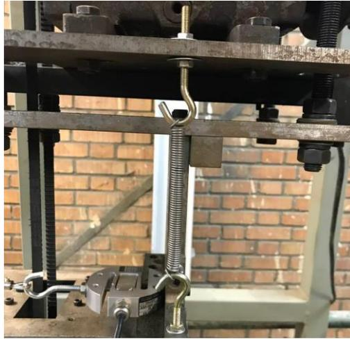
Fig. 3 Primary load mechanism
