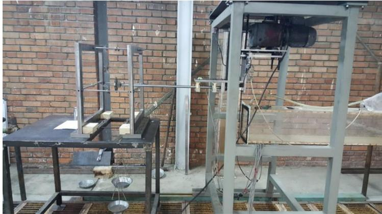
Fig. 6 Propeller model test mechanism calibration system
