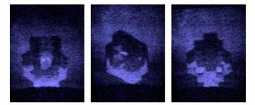
Fig. 1 Appearance of the same object in sonar images changing depending on the viewing angles
