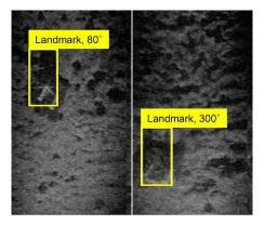
Fig. 13 Shape of landmark in sonar images captured in the sea trials
