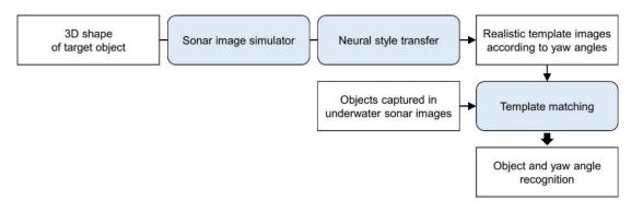
Fig. 2 The proposed method for underwater objects' yaw estimation
