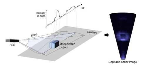
Fig. 3 Imaging mechanism of the FSS
