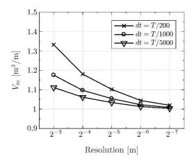
Fig. 4 Investigation of scale resolution and time-step size,  $V_m$  is the total fluid volume flow through the opening of the main reservoir, measured using different scale resolutions and time-step sizes
