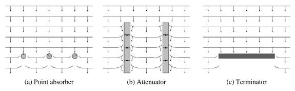
Fig. 1 Schematic illustration of WECs classified by their orientations in wave. The arrows indicate wave direction while the horizontal lines represent incident wavefront
