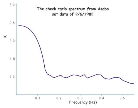
Fig. 1 The check ratio wave spectrum at Asabo
