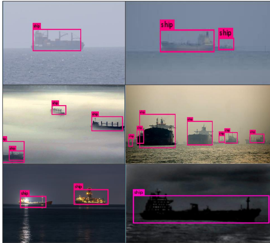
Fig. 19 (Model #3) Ship detection test under low visibility: rain (top), fog (middle), and night (bottom) conditions
