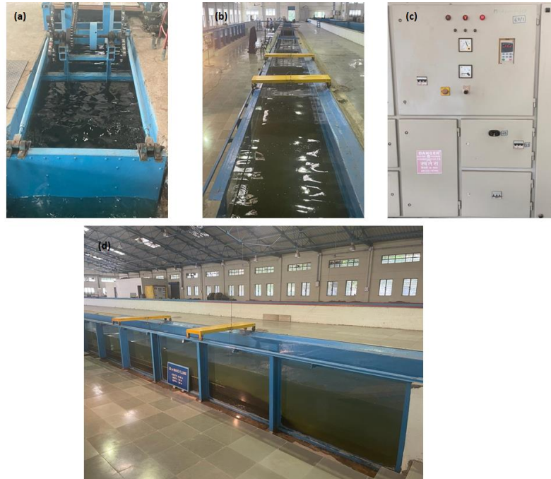
Fig. 7 (a) Flap type paddle, (b) Flap type paddle, (c) Frequency drive and (d) Lengthwise wave flume
