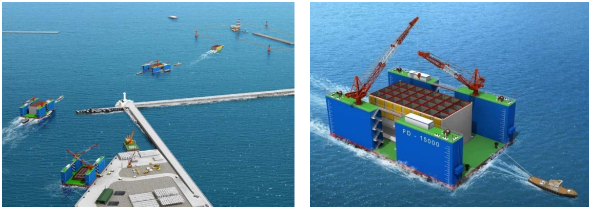
Fig. 2 Schematic view of transferring a caisson on a floating dock
