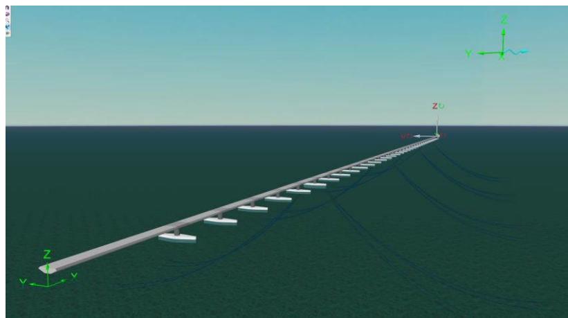
Fig. 4 Straight floating ponton bridge model in OrcaFlex
