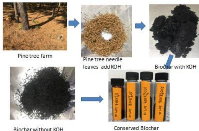
Fig. 1 Schematics of biochar production processes from pine tree needle leaves with KOH
