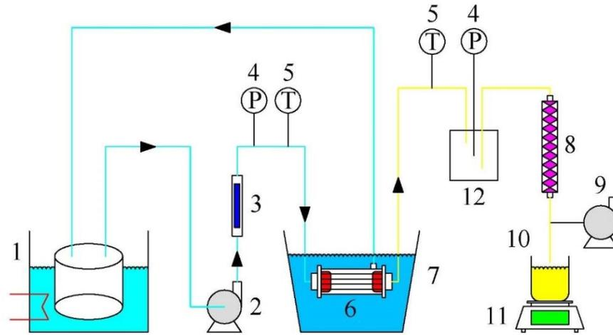
Fig. 1 Flow chart of ultrasonic assisting VMD equipment. 1. Thermostatic water bath; 2. Magnetic drive pump; 3. Liquid flowmeter; 4. Manometer; 5. Thermometer; 6. Hollow fiber membrane module; 7. Ultrasonic cleaning tank; 8. Condenser; 9. Vacuum pump; 10. Product collection tank; 11. Electronic balance; 12. Buffer bottle
