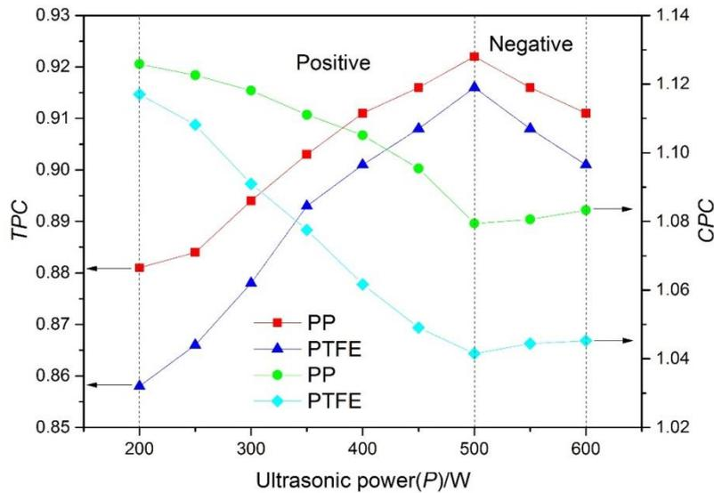
Fig. 13 Effect of ultrasonic power on TPC and CPC
