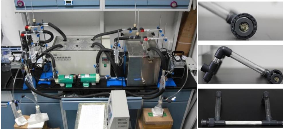
Fig. 2 Photograph of ultrasonic assisting VMD equipment and membrane module
