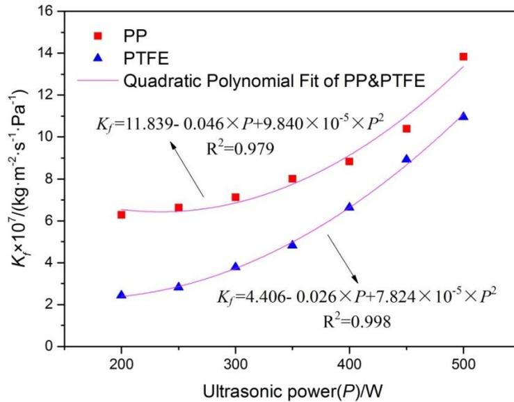
Fig. 10 Relationship between feed side transfer coefficient and ultrasonic power
