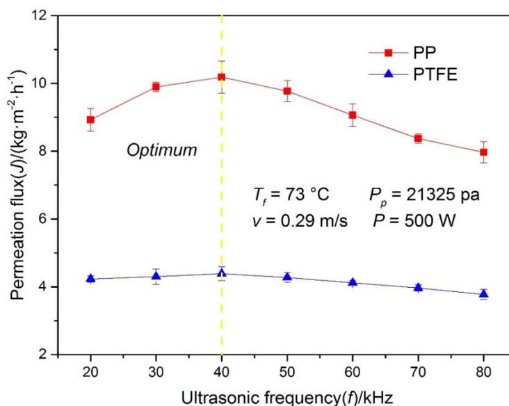
Fig. 7 Effect of the ultrasonic frequency to permeation flux
