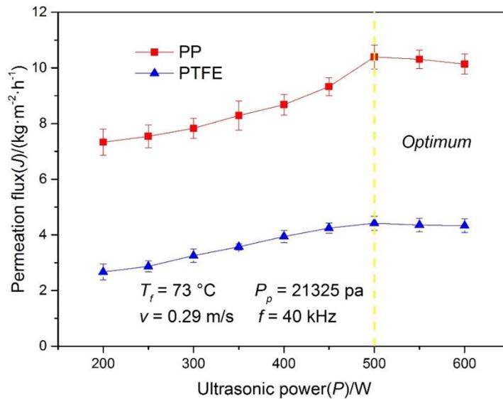
Fig. 6 Effect of the ultrasonic power to permeation flux
