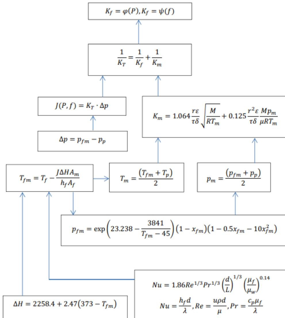
Fig. 8 Calculation flow chart of equations implicit containing only  $K_f$  and  $P$ ,  $K_f$  and  $f$
