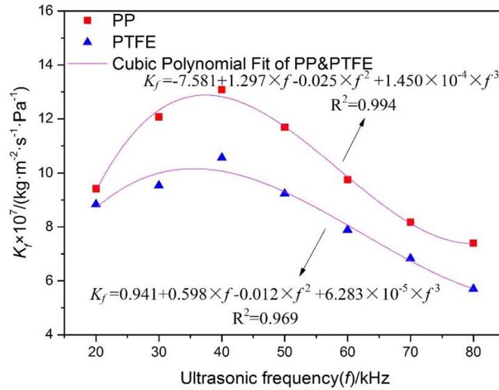
Fig. 12 Relationship between feed side transfer coefficient and ultrasonic frequency
