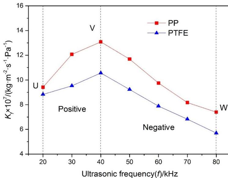
Fig. 11 Effect of ultrasonic frequency to feed side transfer coefficient
