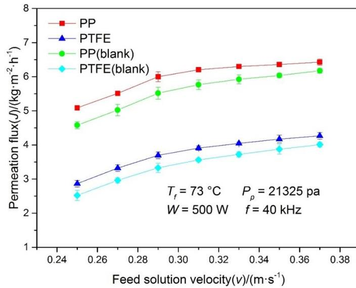
Fig. 5 Effect of the feed solution velocity to permeation flux
