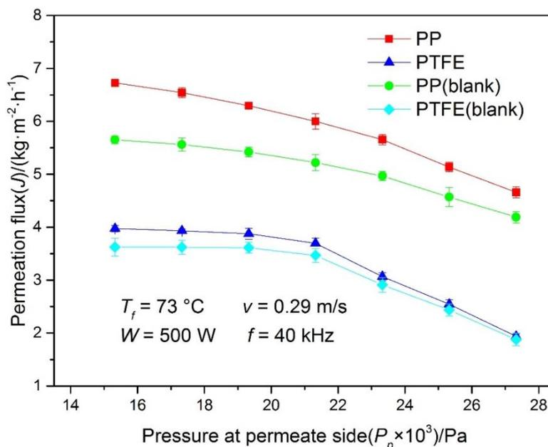
Fig. 4 Effect of the pressure at permeate side to permeation flux
