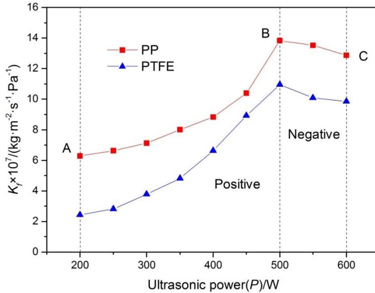
Fig. 9 Effect of ultrasonic power to feed side transfer coefficient
