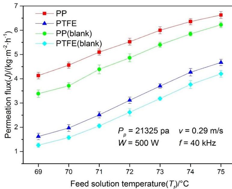
Fig. 3 Effect of the feed solution temperature to permeation flux
