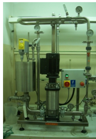
Fig. 1 J.A.M. INOX PRODUKT cross-flow membrane system (1 - feed tank, 2 - pump, 3 - pressure gauge, 4 - thermostat, 5 - flowmeter, 6 - membrane module, 7 - permeate, 8 - concentrate, 9 - permeate tank, 10 - valve)
