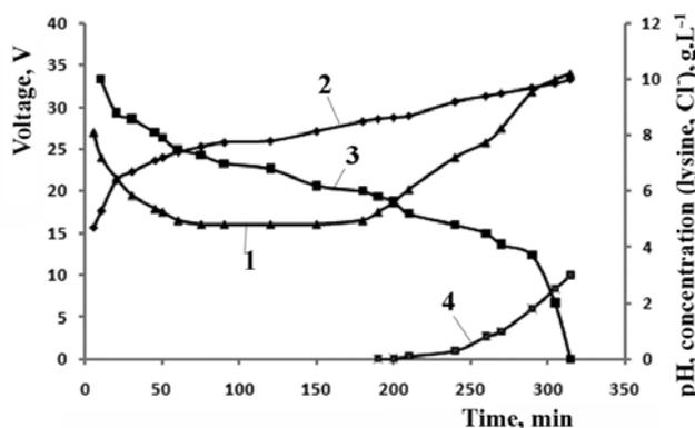
Fig. 2 Changes of voltage in the circuit, pH and concentration of  $\text{Cl}^-$  ions in the lysine solution and the contents of lysine in the water chamber in the process of hydrochloride (concentration  $0.3 \text{ mol.L}^{-1}$ ) transformation into zwitterionic form in a four-chamber electro dialyzer depending on time.
