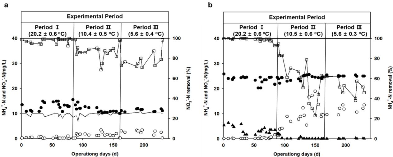
Fig. 3 Ammonium (—), nitrate concentrations in the influent (●) and effluent (○) and nitrate removal (□) in the DPAO SBR (a) and nitrate (▲), ammonium concentrations in the influent (●) and effluent (○) and ammonium removal (□) in PAO SBR (b) long-term operation. DPAO, dinitrifying phosphorus accumulating organisms, and PAO, phosphorus accumulating organisms.
