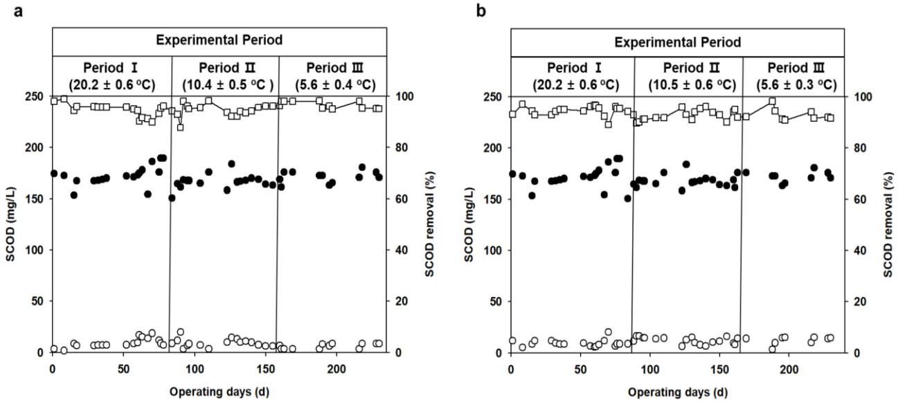
Fig. 1 SCOD concentrations in the influent (●) and effluent (○) and SCOD removal (□) in the long-term operation of the DPAO (a) and PAO (b) SBRs. SCOD, soluble chemical oxygen demand, DPAO, diritrifying phosphorus accumulating organisms, and PAO, phosphorus accumulating organisms.
