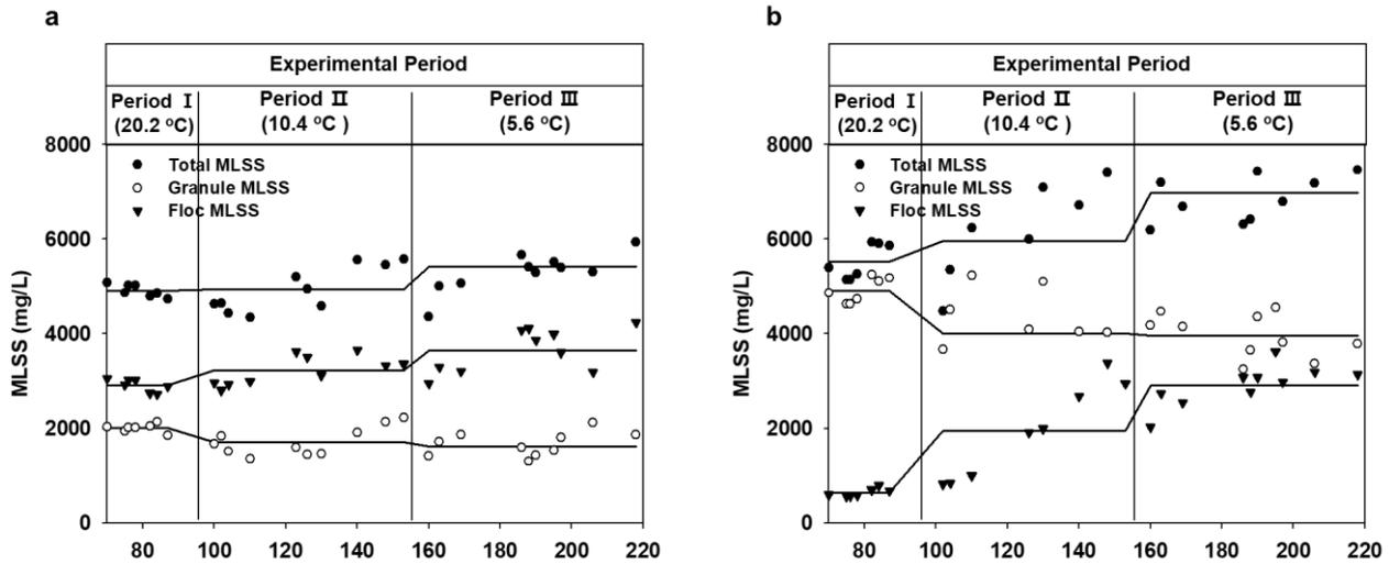
Fig. 5 Flocculent and granular sludge MLSS in the granular DPAO (a) and PAO (b) SBRs at different temperatures. MLSS, mixed liquor suspended solids, DPAO, denitrifying phosphorus accumulating organisms, and PAO, phosphorus accumulating organisms.
