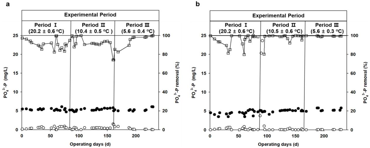
Fig. 2 Phosphate concentrations in the influent (●) and effluent (○) and phosphate removal (□) in the long-term operation of the DPAO (a) and PAO (b) SBRs. DPAO, dinitrifying phosphorus accumulating organisms, and PAO, phosphorus accumulating organisms.
