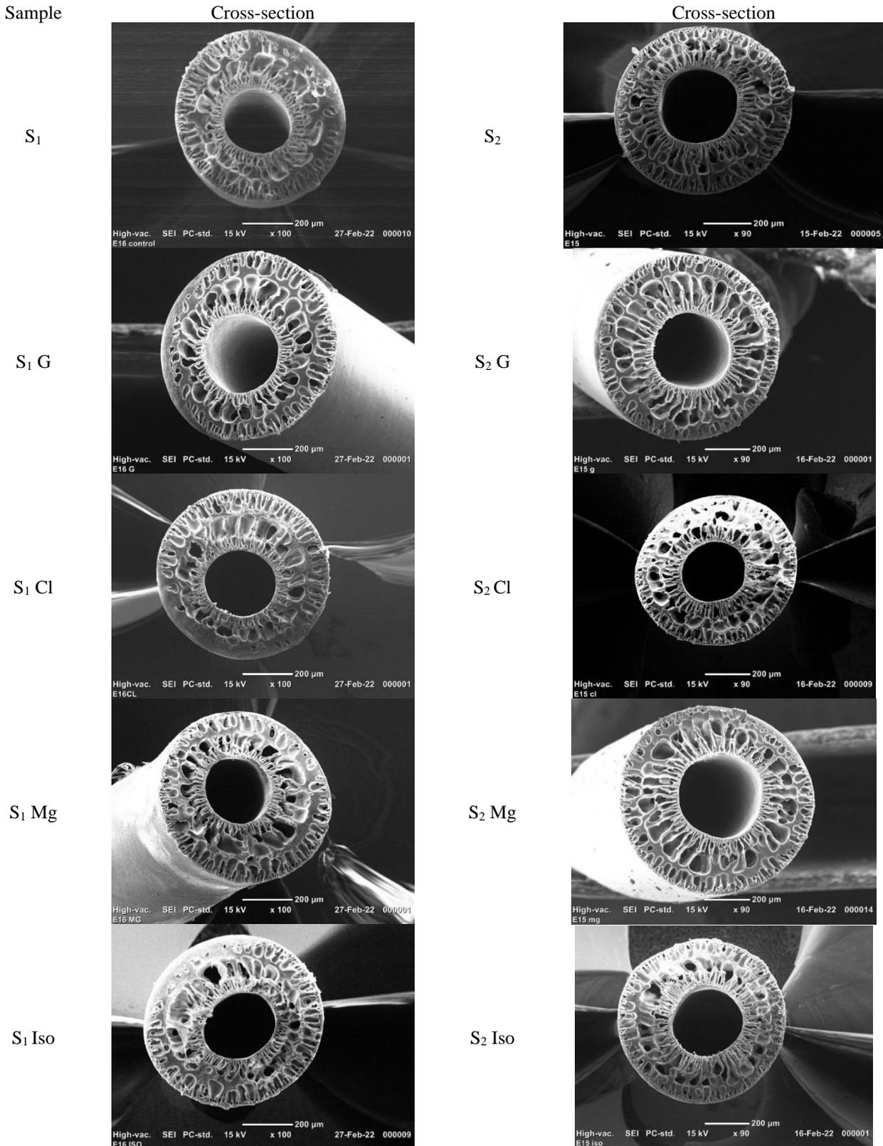
Fig 1 SEM cross-section morphology of pristine and post treated samples with and without TEOS
