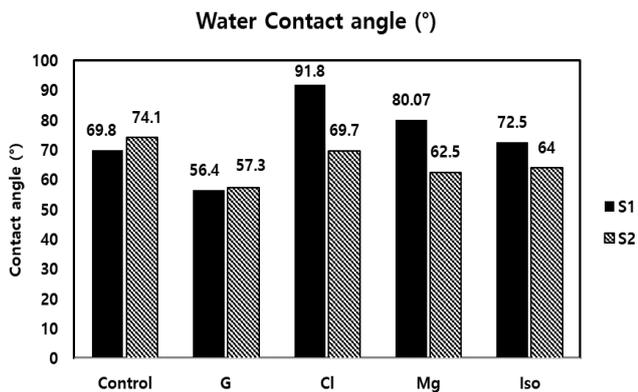
Fig. 3 Water contact angle of pristine and post treated samples with and without TEOS
