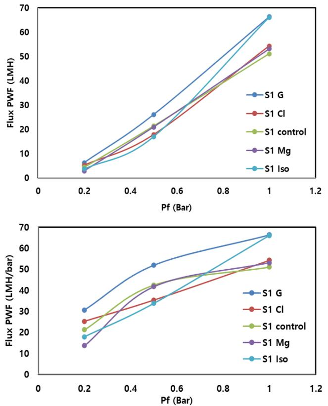
Fig. 4 PWF and PWF/bar (LMH L/m<sup>2</sup>/h and LMH/bar) of pristine and post-treated samples without TEOS
