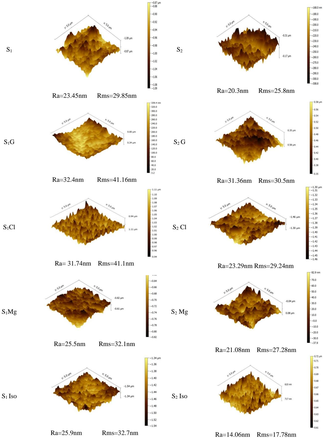
Fig. 2 Surface Roughness: 3D images, Ra (nm) & Rms (nm) of S1, S2, control and post treated samples
