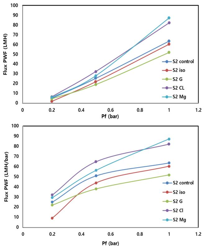
Fig. 5 PWF and PWF/bar (LMH L/m<sup>2</sup>/h and LMH/bar) of pristine and post-treated samples with TEOS
