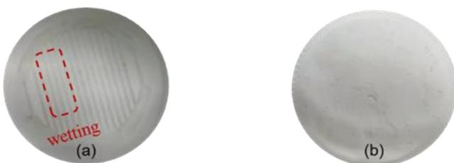
Fig. 14 Surface state of PVDF base membrane (a) and PVDF-PFTS/SiO<sub>2</sub> membrane (b) after DCMD experiment NaCl solution (3.5 wt%) was used as the feed solution
