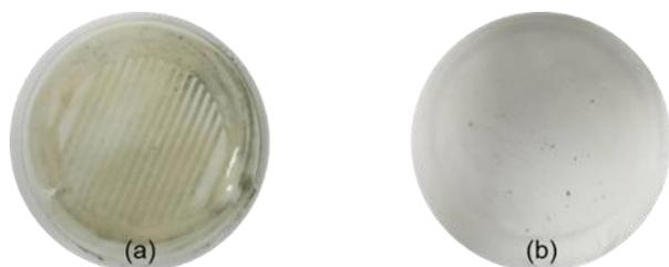
Fig. 16 Simulated oily high-salt wastewater was used as the feed solution, the surface state of PVDF base membrane(a) and PVDF-PFTS/SiO<sub>2</sub> membrane(b) after DCMD experiment
