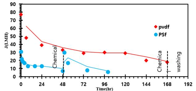
Fig. 5 Permeate flux for both MBR
