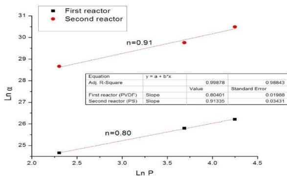
Fig. 4 Compressibility coefficient in both MBR
