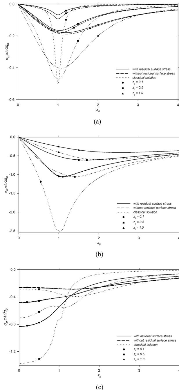
Fig. 3 Non-dimensional stress profiles of a half-plane under horizontal surface load: (a) Vertical stress, (b) Horizontal stress, (c) Shear stress
