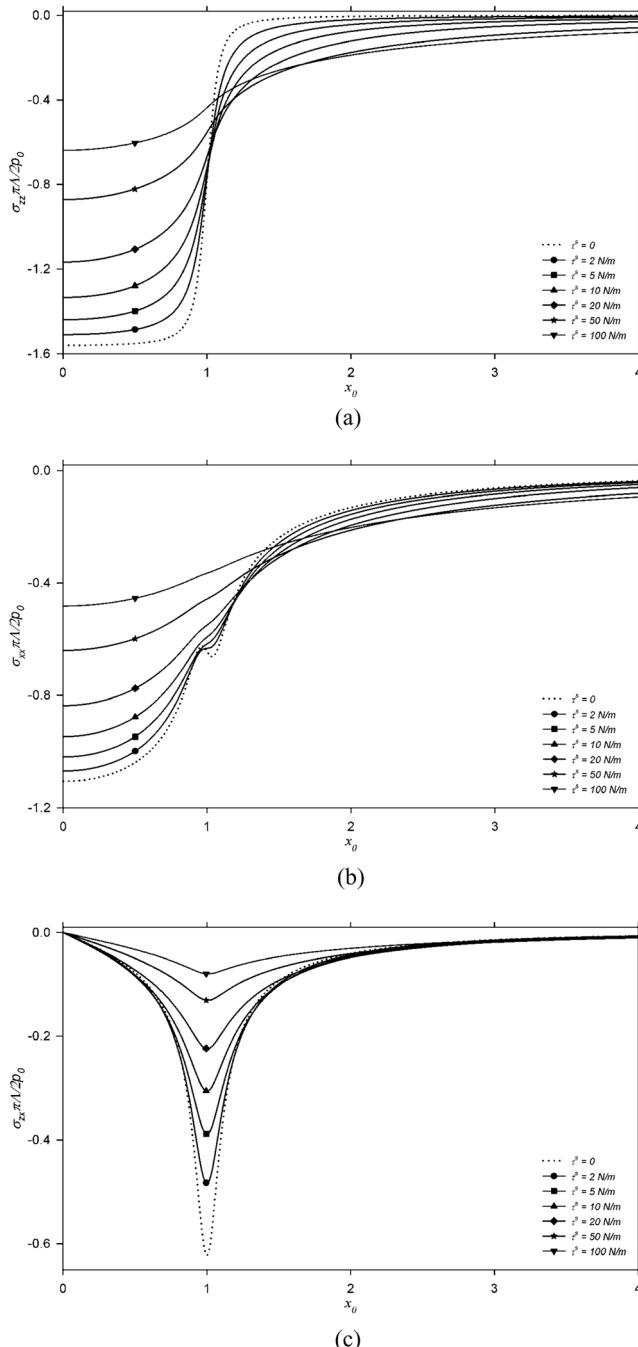
Fig. 5 Non-dimensional stress profiles at  $z_0 = 0.1$  under vertical surface load for different residual surface stresses: (a) Vertical stress, (b) Horizontal stress, (c) Shear stress
