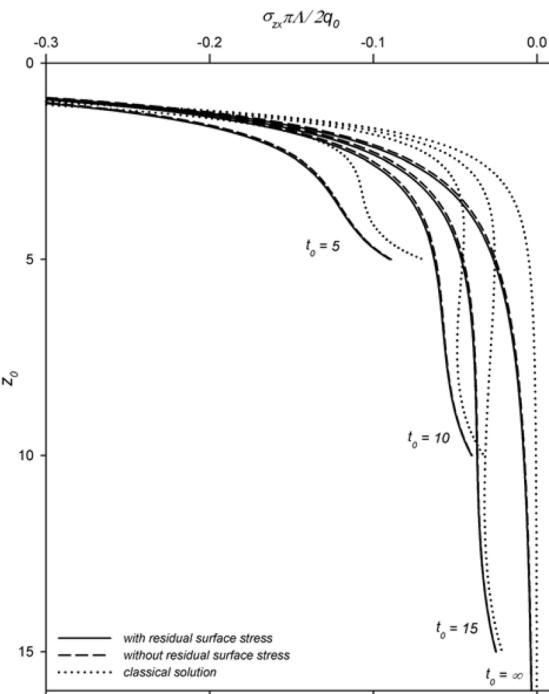
Fig. 9 Non-dimensional shear stress along the  $z$ -axis of a finite layer under horizontal surface load
