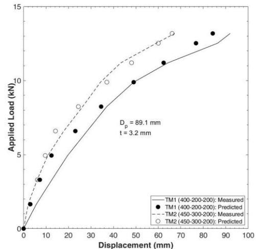
Fig. 21 Predicted versus field test data for TM1 & TM2
