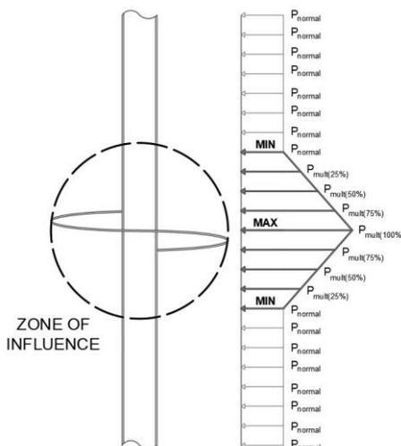
Fig. 18 Distribution of *p*-multipliers on the *p-y* springs for helical piles
