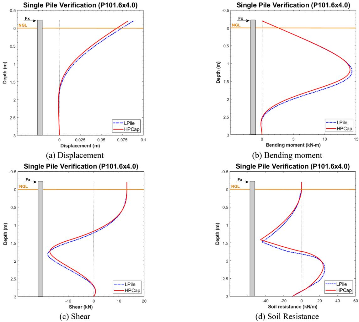
Fig. 14 Comparative results between HPCap and LPile in establishing validity
