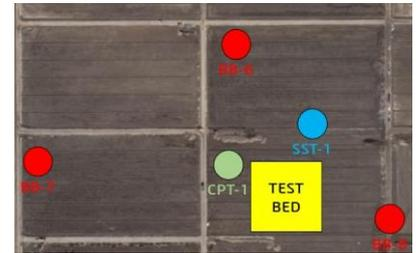
(c) Location of CPT, SPT and SST relative to test bed
