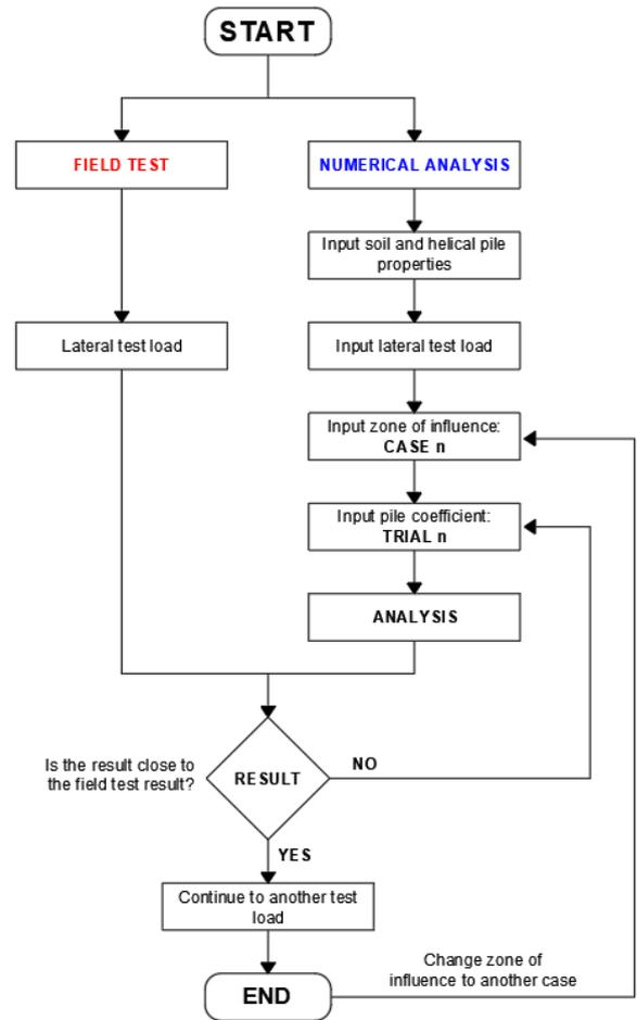
Fig. 19 Reiterative process flow for determination of pile coefficient and zone of influence
