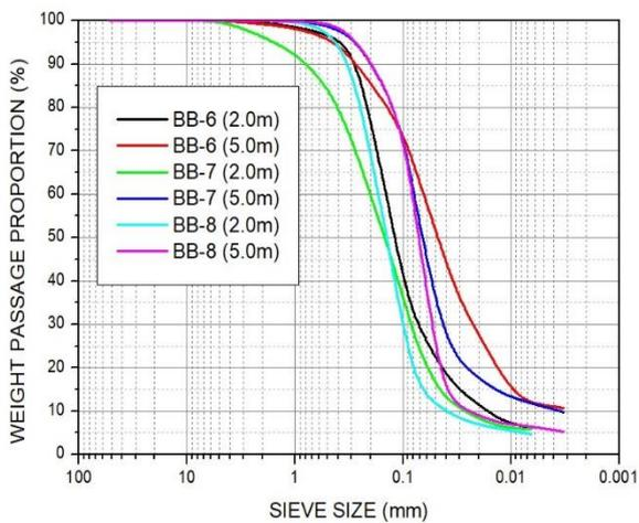
Fig. 12 Particle size distribution curve for BB-6, BB-7 and BB-8
