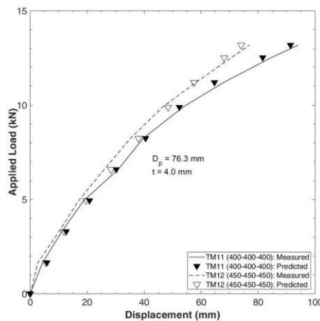
Fig. 24 Predicted versus field test data for pile with  $D_p = 76.3$  mm
