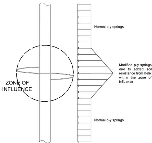
Fig. 17 Distribution of *p-y* springs for helical piles
