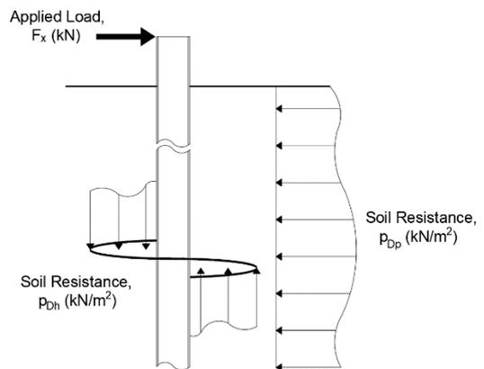
Fig. 15 Soil resistance concept for laterally loaded helical piles
