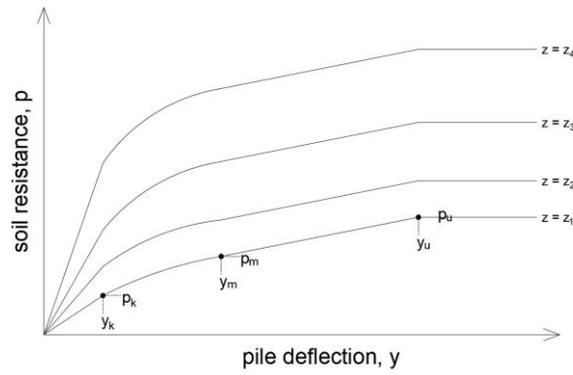
Fig. 3 Characteristic shape of a  $p$ - $y$  curve for sandy soils
