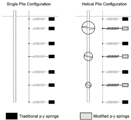
Fig. 16 Comparison between a single pile versus a helical pile *p-y* spring configuration
