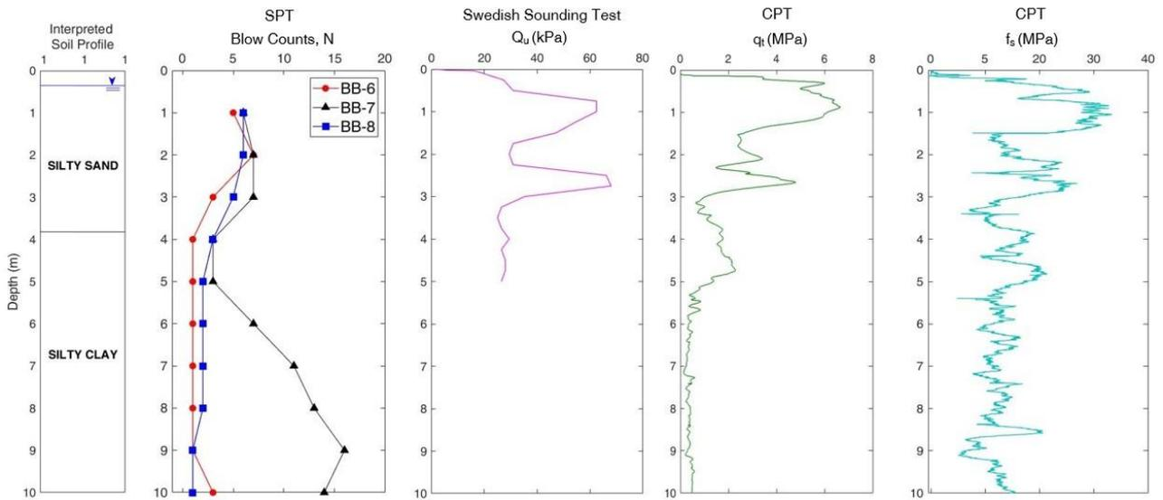
Fig. 11 Collected soil data from various in-situ tests
