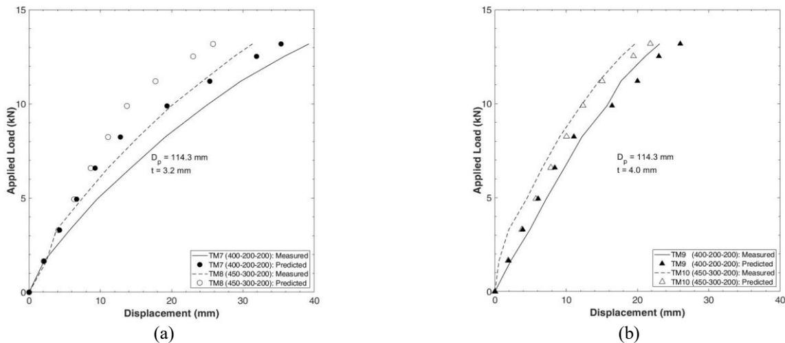
Fig. 23 Predicted versus measured data for piles with  $D_p = 114.3$  mm (a) TM7 & TM8 and (b) TM9 & TM10
