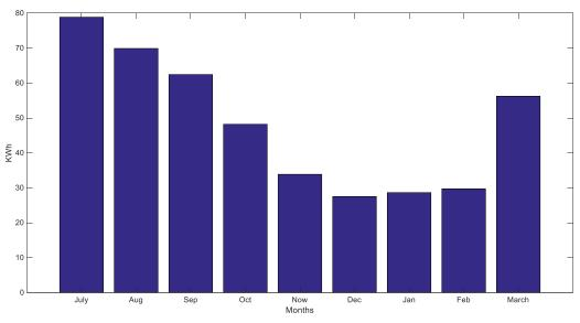
Fig. 7 Monthly energy production of the PV system from July 2018 to March 2019
