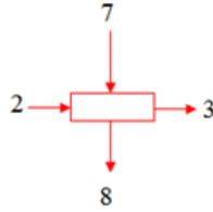
The rate at which exergy losses taken place in condensation process may be formulate as,
