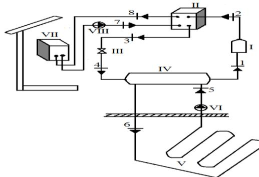
Fig. 1 Graphical layout of proposed system for heating mode. (I) Compressor (II) Condenser (III) Capillary tube (IV) Evaporator (V) Earth heat exchanger (VI) Water circulating pump
