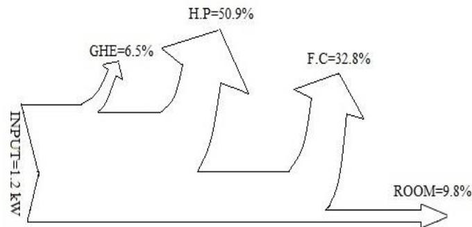
Fig. 2 Exergy flow diagram of GSHP System
