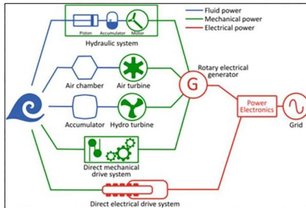
Fig. 4 Different paths for electricity conversion from wave energy (Pecher and Kofoed 2016)
