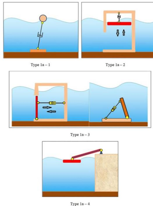
Fig. 6 Tethered WECs of the Type 1
