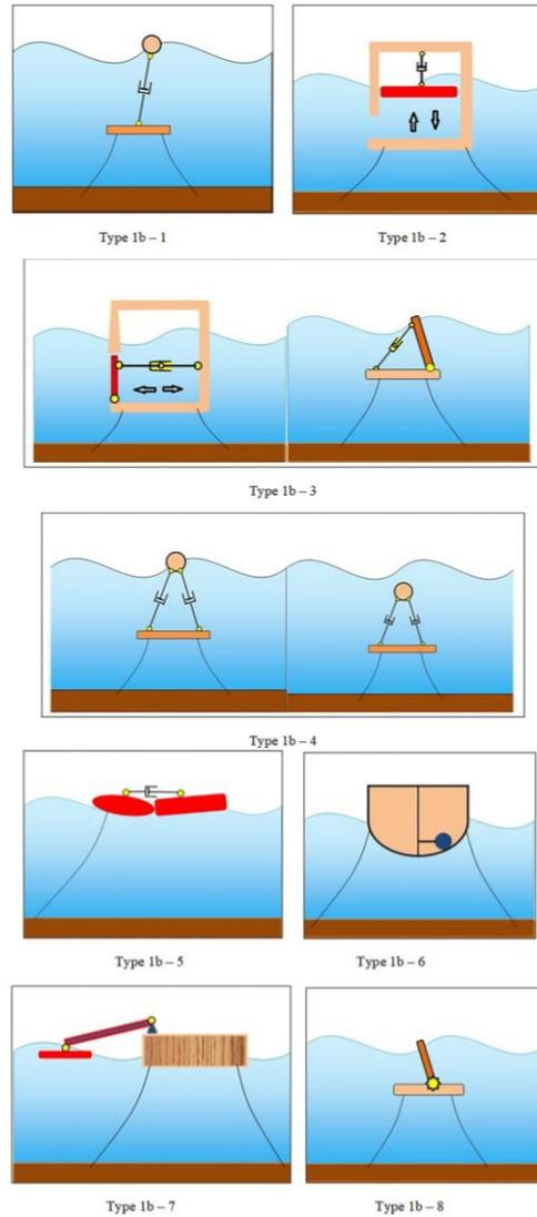
Fig. 7 Floating WECs of the Type 1
