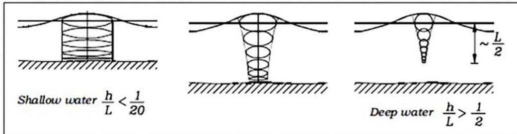
Fig. 3 Movement of water molecules according to the water depth (Andersen and Frigaard 2011)
