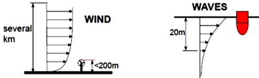
Fig. 1 Comparison of the velocity profiles of the wave and wind (Falcão 2010)
