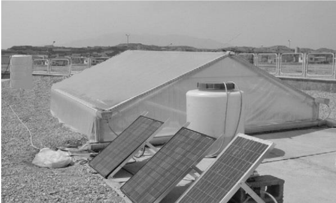
Fig. 1 The photograph of used closed solar powered still
