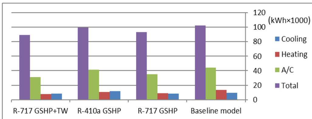
Fig. 3 The annual energy consumption of baseline model and three retrofitting scenarios in four subdivide energy demand sections
