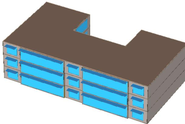
Fig. 2 Trombe walls and the overhangs on the south façade of the building in the eQuest model
