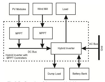
Fig. 2 Configuration of the proposed hybrid power system
