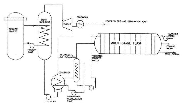
Fig. 1 Schematic illustration of a simple desalination nuclear reactor circuit (Majumdar 2002)
