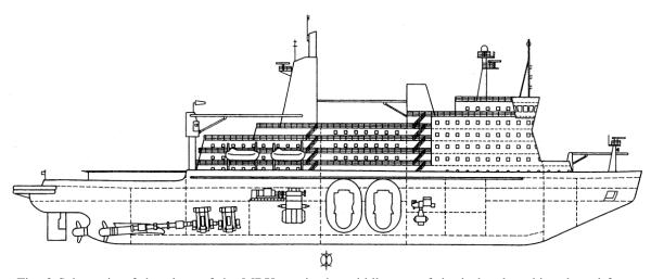
Fig. 3 Schematic of the place of the MRX put in the middle part of the icebreaker ship adapted from Kusunoki (2000)
