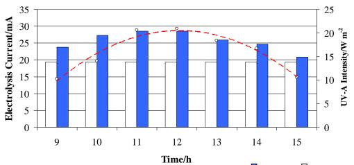
Fig. 8 Electrolysis current vs time with direct solar exposition ( $\Box$ ) or dark ( $\Box$ ) and UV-A intensity (- $\circ$ -) in KOH 1 M at 25 °C at 1.6 Volt
