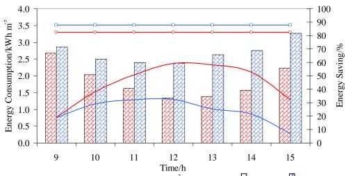
Fig. 9 Photo-electrolyser energy consumption for  $m^3$  of  $H_2$  at 1.5 V ( $\square$ ) or 1.6 V ( $\square$ ) under direct solar exposition and relative energy saving (– or –). Dashed lines represent the energy consumption in dark at 1.5 V (3.29 kWh  $m^{-3}$ ) (- $\square$ -) and at 1.6 V (3.51 kWh  $m^{-3}$ ) (- $\square$ -)
