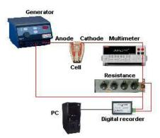
Fig. 1 Scheme of anodization system
