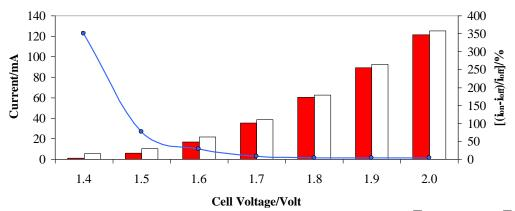
Fig. 5 Current density vs cell voltage with nickel-TiO<sub>2</sub>/Ti anode at UV-on ( $\Box$ ) and UV-off ( $\Box$ ) and relative change of current density (-•-) in KOH 1 M at 25 °C, UV intensity 62 W m<sup>-2</sup>
