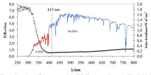
Fig. 4 Absorption coefficient spectra of the  $TiO_2/Ti$  ( $\circ$ ) according to the Kubelka-Munk equation and global solar irradiance in UV (-) or Visible (-) (Grimes *et al.* 2008)
