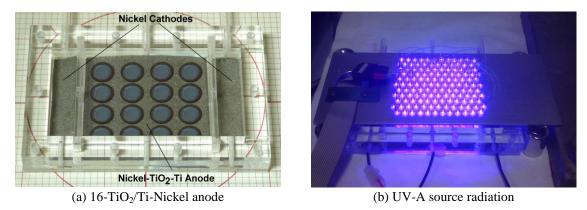
Fig. 2 Photo-electrolysis cell
