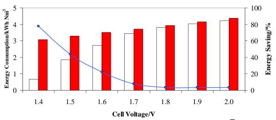
Fig. 6 Energy consumption vs cell voltage with Nickel-TiO<sub>2</sub>/Ti anode at UV-on ( $\Box$ ) and UV-off ( $\Box$ ) and relative energy saving (-•-) in KOH 1 M at 25°C, UV intensity 62 W m<sup>-2</sup>
