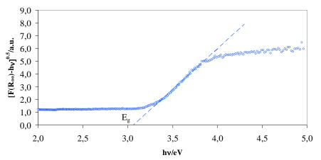
Fig. 3 The transformed Kubelka-Munk function vs. energy of excitation source for TiO<sub>2</sub>/Ti (0)
