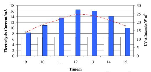
Fig. 7 Electrolysis current vs time with direct solar exposition ( $\Box$ ) or dark ( $\Box$ ) and UV-A intensity (- $\circ$ -) in KOH 1 M at 25°C at 1.5 Volt
