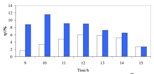
Fig. 10 Solar conversion efficiency vs time with direct solar exposition at 1.5 V( $\Box$ ) and 1.6 V dark ( $\Box$ )in KOH 1 M at 25 °C
