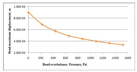
Fig. 3 Variation of displacement vs. overbalance pressure in bend area for a sidetrack with  $45^{\circ}$  inclination from the vertical direction and the direction along  $\sigma$ h in NF-SS stress regime
