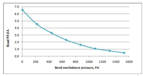
Fig. 2 Variation of NYZA vs. overbalance pressure in bend area for a sidetrack with  $45^{\circ}$  inclination from the vertical direction and the direction along  $\sigma$ h in NF-SS stress regime
