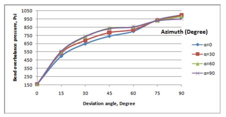
Fig. 5 Minimum overbalance pressure vs. sidetrack orientation in NF stress regime
