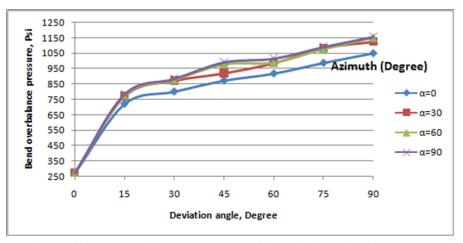
Fig. 7 Minimum overbalance pressure vs. sidetrack orientation in SS stress regime
