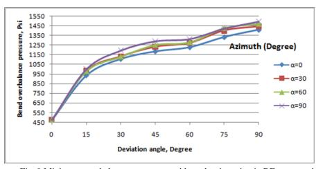
Fig. 9 Minimum overbalance pressure vs. sidetrack orientation in RF stress regime
