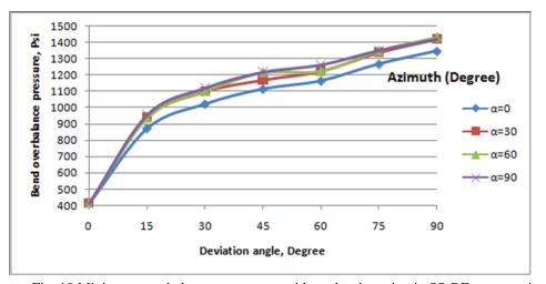
Fig. 10 Minimum overbalance pressure vs. sidetrack orientation in SS-RF stress regime
