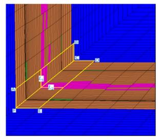
Fig. 1 Schematic view of the bend area and the surrounding plastic zone
