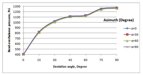
Fig. 4 Minimum overbalance pressure vs. sidetrack orientation in hydrostatic stress regime
