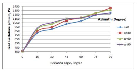
Fig. 8 Minimum overbalance pressure vs. sidetrack orientation in NF-SS stress regime
