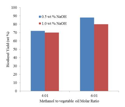
Fig. 3 Influence of Catalyst Concentration on the yield of Biodiesel (at 30°C reaction temperature and 30 minutes reaction time)
