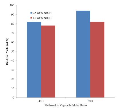
Fig. 1 Influence of Molar Ratio of Methanol to Oil on the yield of Biodiesel (at 30°C and 60 minutes) reaction
