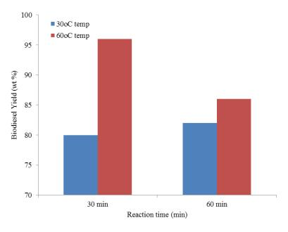
Fig. 2 Influence of Temperature on the yield of Biodiesel (at 6:1 Molar ratio and 1.0 wt % NaOH)
