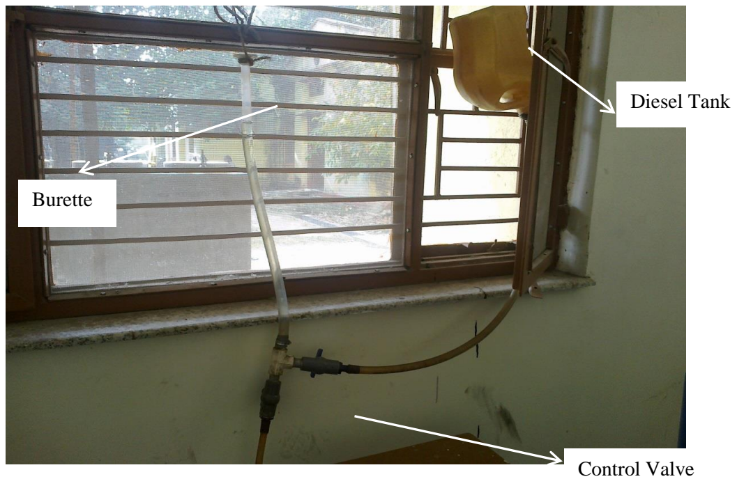
Fig. 4 Fuel feed setup
