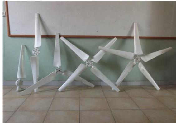
Fig. 7 Turbines used in the solar chimney power plant ( $r=0.4$  m)
