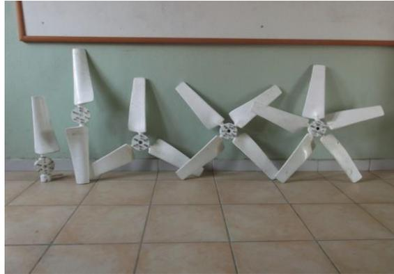
Fig. 6 Turbines used in the solar chimney power plant ( $r=0.4$  m)
