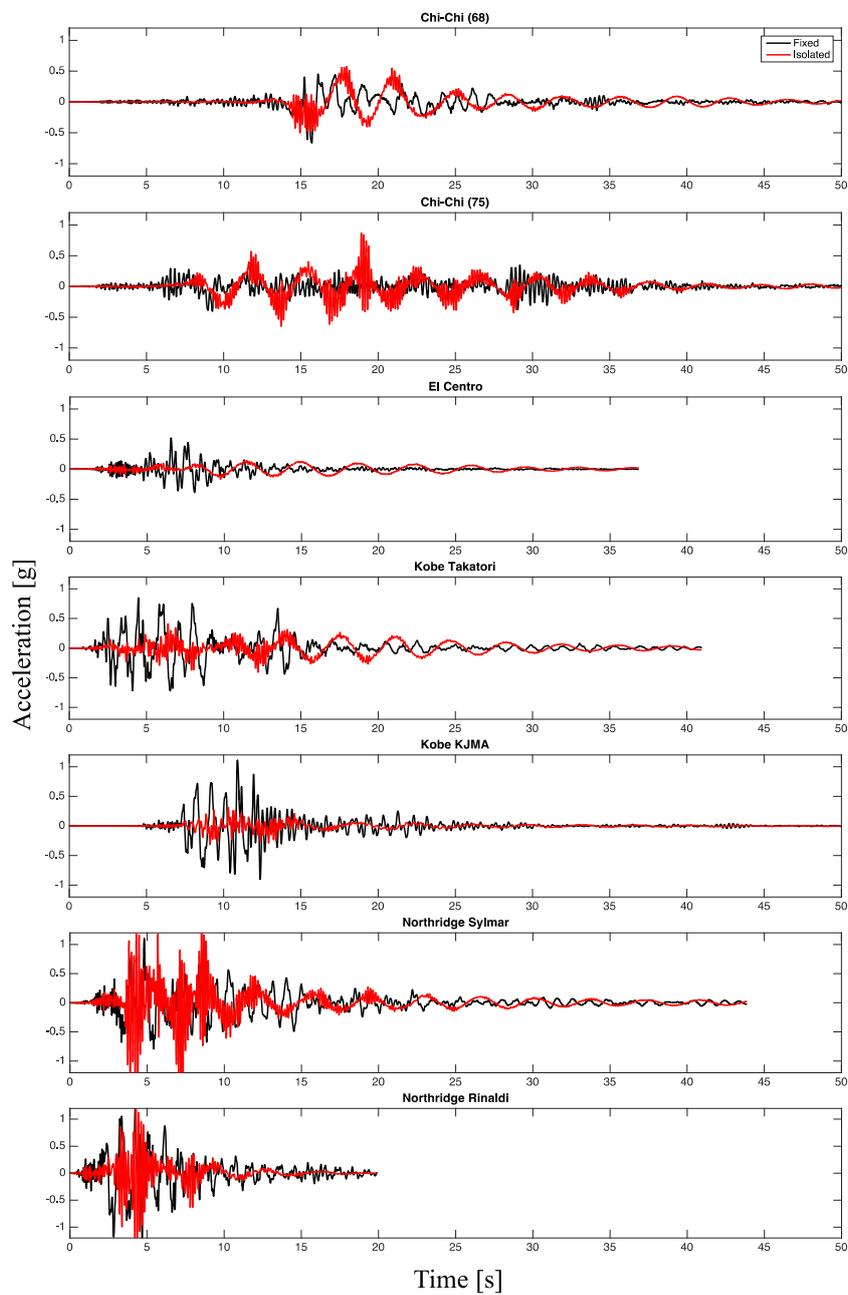
Fig. 6 Horizontal absolute acceleration time histories for fault parallel biaxial ground motions at the 2nd floor
