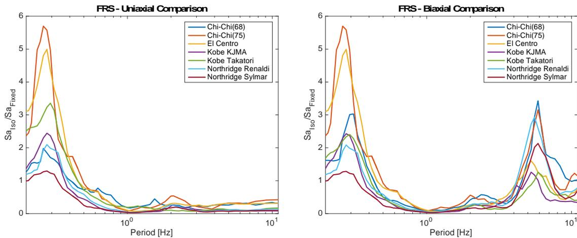
Fig. 10 Ratios of isolated to fixed based horizontal floor response spectra for uniaxial (left) and biaxial (right) fault normal motions at the roof level
