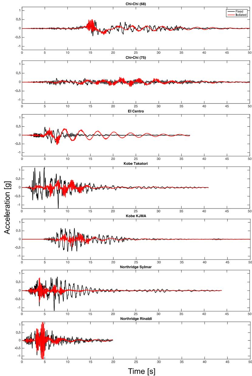
Fig. 7 Horizontal absolute acceleration time histories for fault normal biaxial ground motions at the 2nd floor
