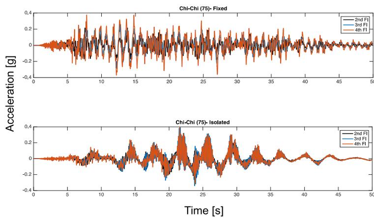
Fig. 8 Horizontal absolute acceleration time histories for Chi-Chi (75) fault normal biaxial ground motions at all floors for the fixed (top) and isolated
