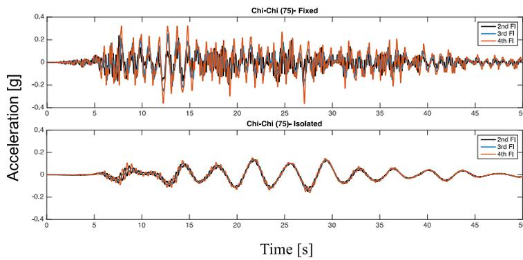
Fig. 4 Horizontal absolute acceleration time histories for Chi-Chi (75) fault normal uniaxial ground motions at all floors for the fixed (top) and isolated
