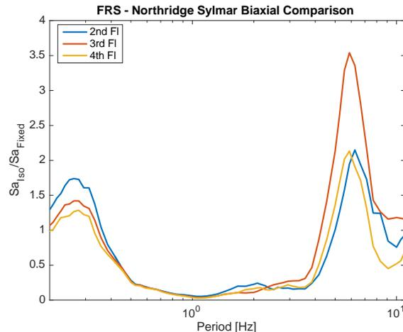
Fig. 11 Ratios of isolated to fixed based horizontal floor response spectra for northridge sylmar biaxial (right) fault normal motions at all levels
