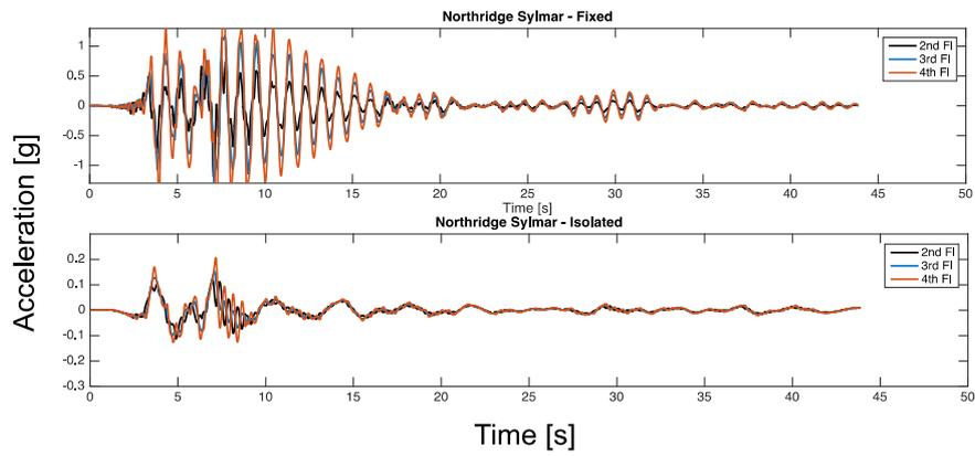
Fig. 5 Horizontal absolute acceleration time histories for northridge sylmar fault normal uniaxial ground motions at all floors for the fixed (top) and isolated
