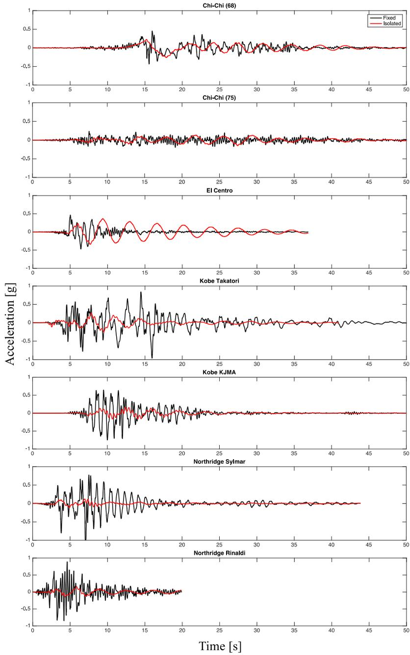
Fig. 3 Horizontal absolute acceleration time histories for fault normal uniaxial ground motions at the 2nd floor
