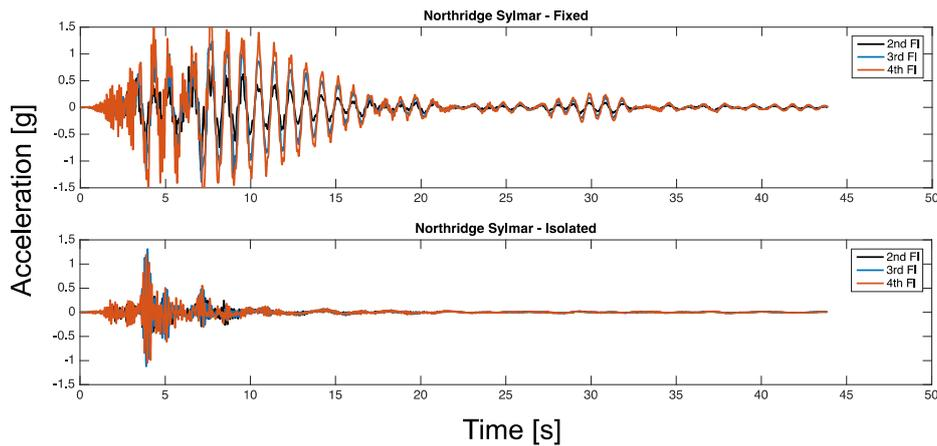
Fig. 9 Horizontal absolute acceleration time histories for northridge sylmar fault normal biaxial ground motions at all floors for the fixed (top) and isolated
