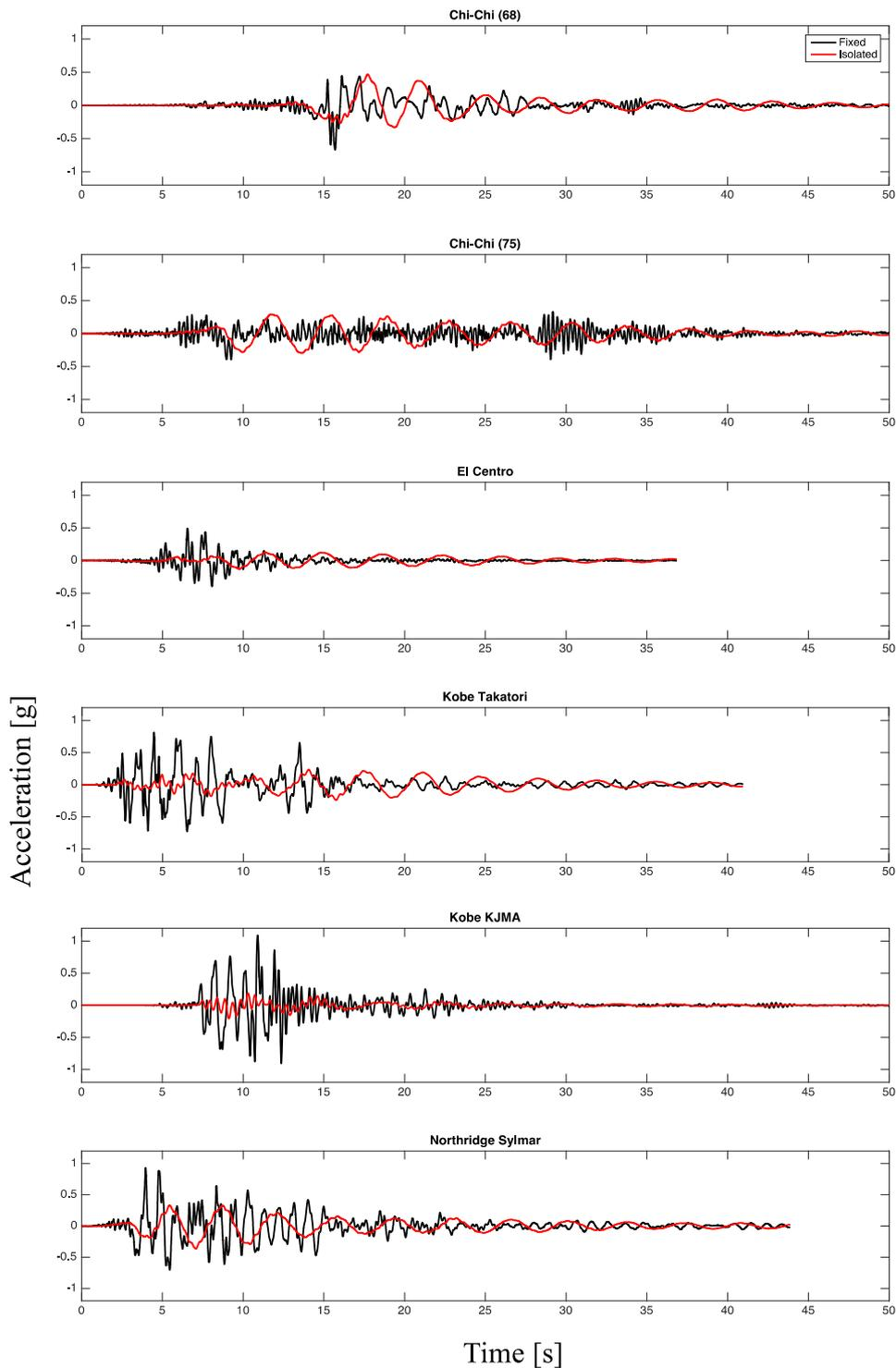
Fig. 2 Horizontal absolute acceleration time histories for fault parallel uniaxial ground motions at the 2nd floor
