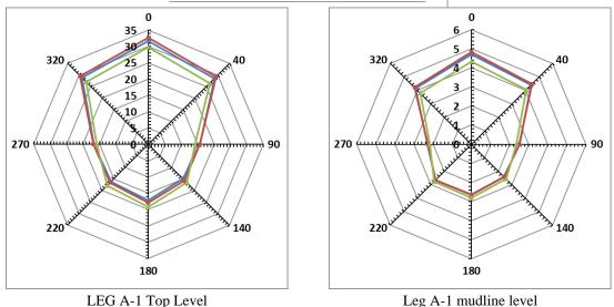
Fig. 9 Absolute horizontal displacement for extreme-2 storm condition for different incidence angles
