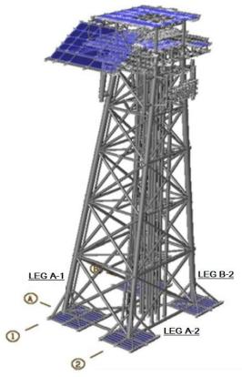
Fig, 4 3D finite element model of the substructure and topside
