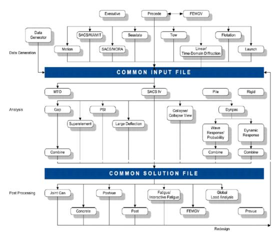
Fig. 5 Modelling, analysis procedure for in-place behavior of the platform based on SACS program
