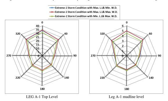
Fig. 8 Absolute horizontal displacement for extreme-1 storm condition for different incidence angles
