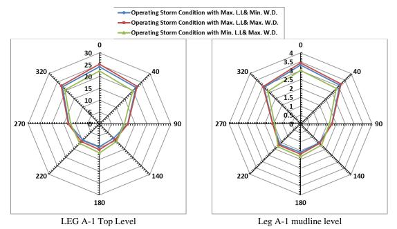
Fig. 7 Absolute horizontal displacement for operating storm condition for different incidence angles
