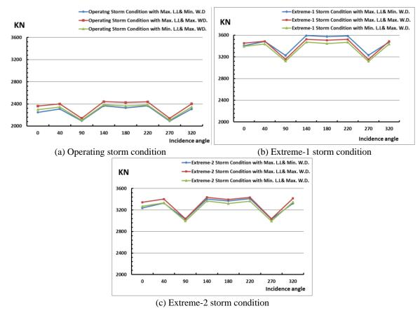
Fig. 6 Total applied horizontal loads for different incidence angles of the environmental loads' direction
