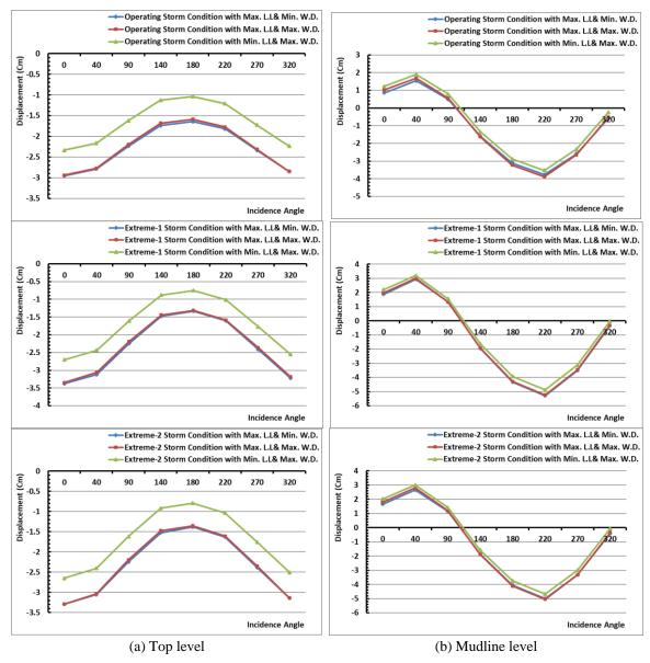
Fig. 10 Vertical displacement for top level (left) and mudline level (right) of (leg A-1) for three storm conditions according to the angles of the environmental loads' directions
