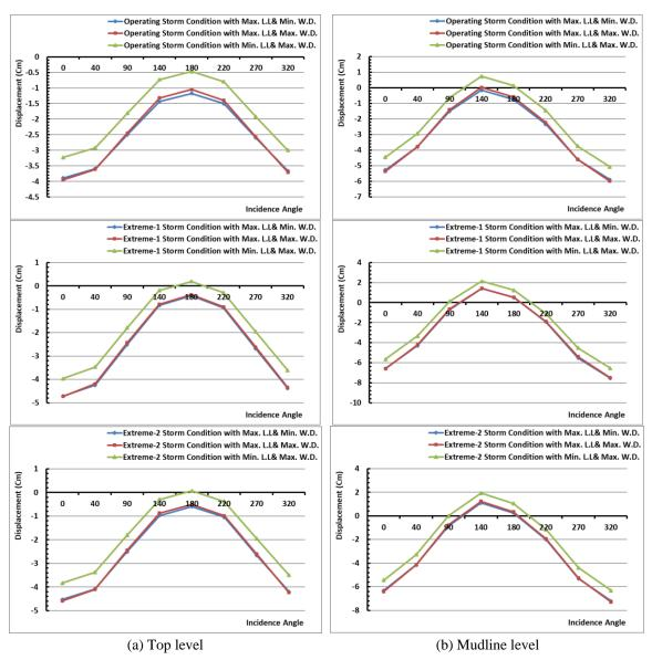
Fig. 11 Vertical displacement for top level (left) and mudline level (right) of (leg A-2) for three storm conditions according to the angles of the environmental loads' directions
