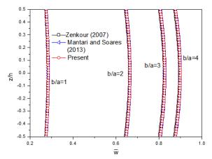
Fig. 5 Distribution of non-dimensional transverse displacement ( $\overline{w}$ ), through the thickness of a thick EG plate (a/h=4, p=0.5)
