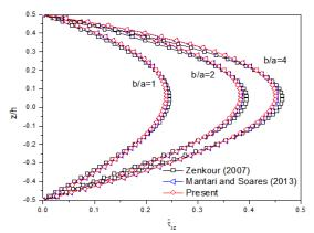
Fig. 8 Distribution of non-dimensional transverse shear stress  $(\bar{\tau}_{xz})$ , through the thickness of a thick EG plate (a/h=4, p=0.5)
