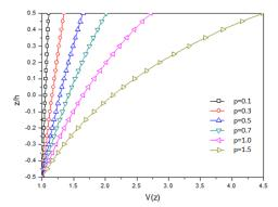
Fig. 2 Exponential function V(z) along the thickness of an EG plate for various values of the parameter p
