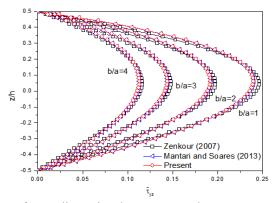
Fig. 9 Distribution of non-dimensional transverse shear stress  $(\bar{\tau}_{yz})$ , through the thickness of a thick EG plate (*a/h*=4, *p*=0.5)
