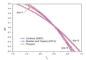
Fig. 7 Distribution of non-dimensional inplane shear stress  $(\bar{\tau}_{xy})$ , through the thickness of a thick EG plate (*a*/*h*=4, *p*=0.5)
