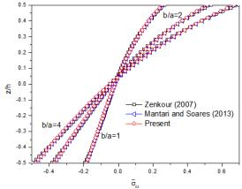
Fig. 6 Distribution of non-dimensional axial stress  $(\overline{\sigma}_{xx})$ , through the thickness of a thick EG plate (a/h=4, p=0.5)
