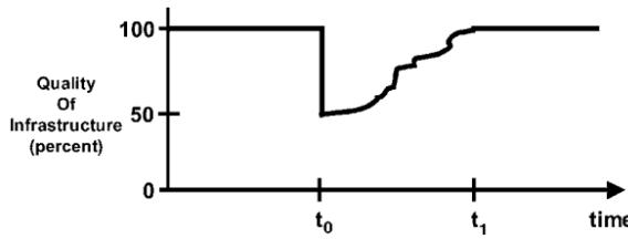
Fig. 4 Schematic representation of seismic resilience concept (Bruneau *et al.* 2003)
