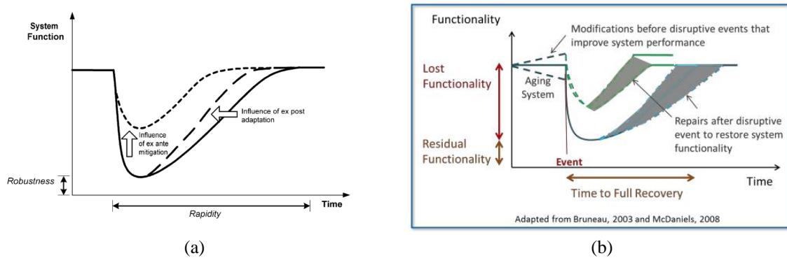
Fig. 7 Effects of decision-making on resilience (McDaniels *et al.* 2008) (McAllister 2013)
