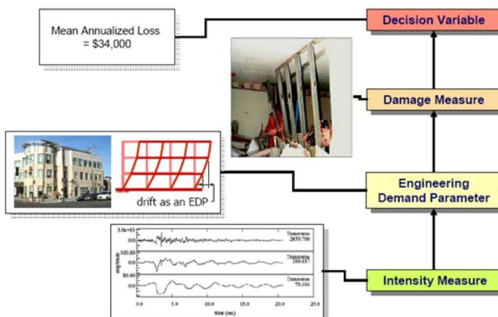
Fig. 1 PEER center methodology for Performance-Based Design (PBD)
