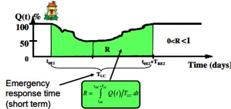
Fig. 5 Functionality curve and resilience (Renschler *et al.* 2010)
