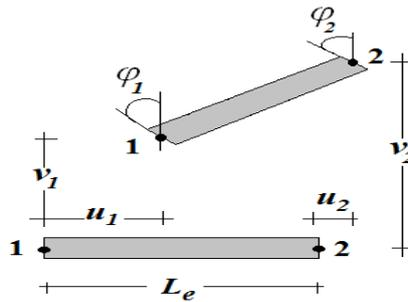
Fig. 3 Finite beam element model
