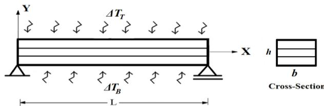
Fig. 1 A simply supported laminated beam subjected to non-uniform temperature rising and cross-section
