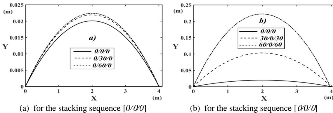
Fig. 5 Thermal nonlinear deflected configuration of the laminated beam for different values of the fiber orientation angles for  $\Delta T_B=500$   $^{\circ}C$
