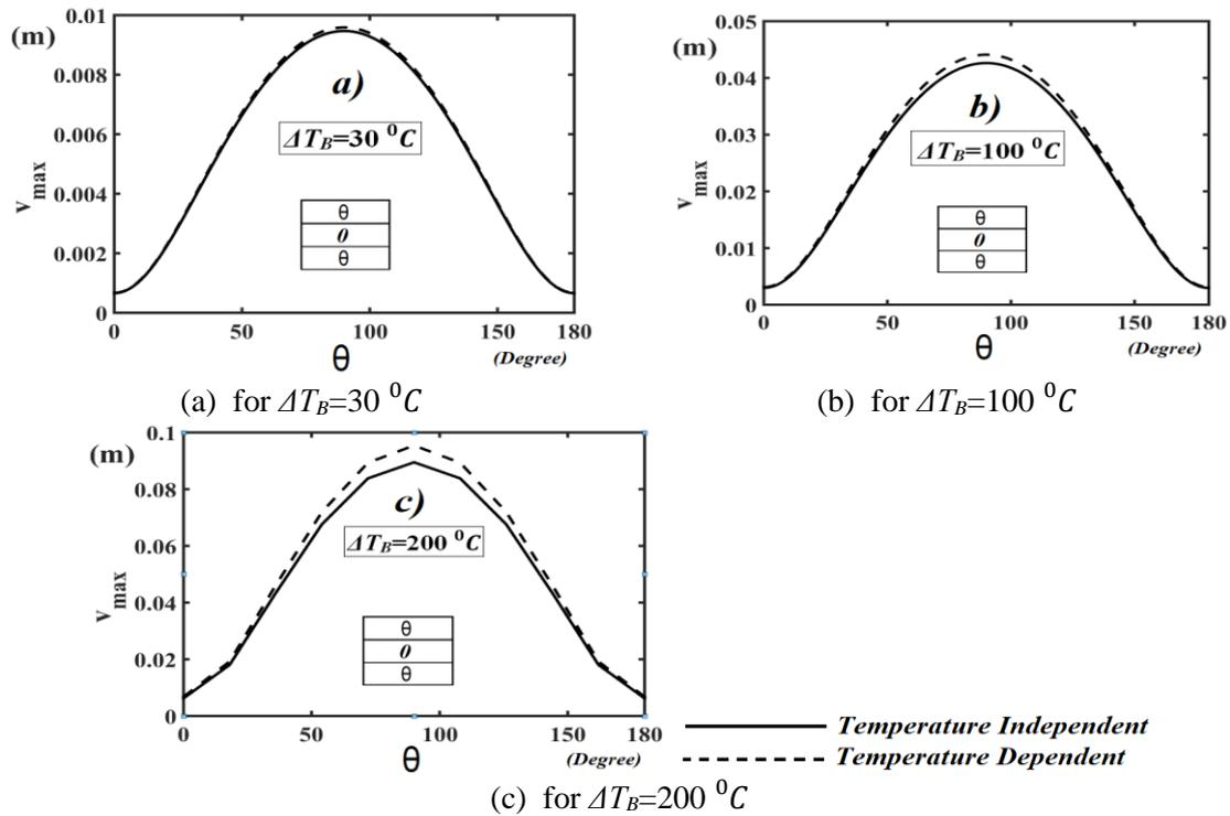
Fig. 7 The relationship between fiber orientation angles and maximum deflections for linear and nonlinear solution for the stacking sequence  $[\theta/\theta/\theta]$
