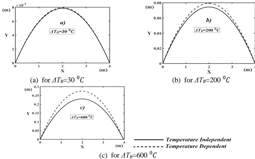
Fig. 8 The difference between temperature dependent and independent physical properties on the nonlinear deflected configuration for the stacking sequence 30/0/30
