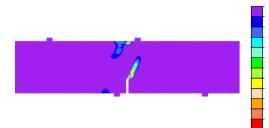
(b) Crack trajectory at the end of simulation time (Newmark scheme)
