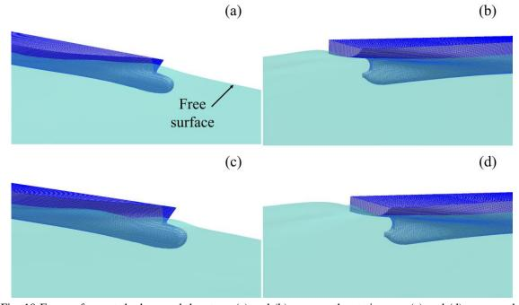
Fig. 10 Free surfaces at the bow and the stern. (a) and (b) concern the static case. (c) and (d) concern the dynamic case
