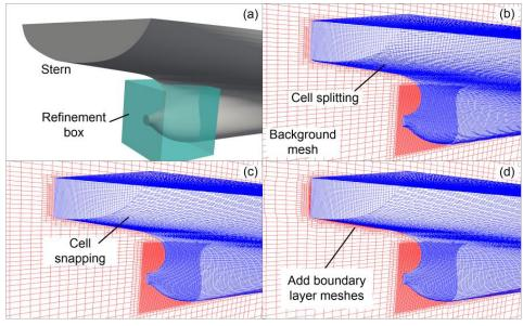
Fig. 4 Mesh generation procedures
