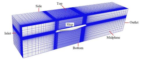
Fig. 3 Computational domain and boundary conditions
