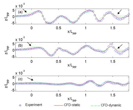
Fig. 9 Wave elevations at the lateral positions (a)  $y/L_{PP}=0.0741$ ; (b)  $y/L_{PP}=0.1509$ ; (c)  $y/L_{PP}=0.4224$ . The arrows point to the differences between the dynamic and static cases. The position values are normalized using the ship length ( $L_{PP}$ ). Experimental data comes from Hino (2005)
