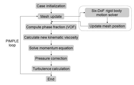
Fig. 1 Flowchart of the solution procedure
