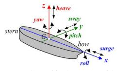
Fig. 2 6-DoF (degree of freedom) motions of the ship
