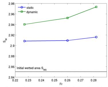
Fig. 12 Comparison of the wetted area ( $S_W$ ) on the hull surface in the static and dynamic cases. Fr is the Froude number.  $S_{W0}$  is the initial wetted area
