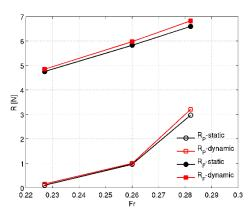
Fig. 14 Pressure  $(R_P)$  and frictional  $(R_F)$  resistances against the Froude number (Fr)
