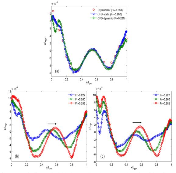
Fig. 11 Wave elevations on the hull surface. (a) Comparison between the static and dynamic cases (Fr=0.260); (b) wave elevations at three Froude numbers in the static case; (c) wave elevations at three Froude numbers in the dynamic case. The arrow points to the changing of the extrema of ship waves. Experimental data comes from Hino (2005). The position values are normalized using the ship length
