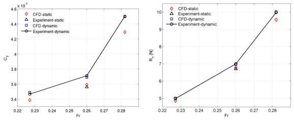
Fig. 13 Total resistance against the Froude number (Fr).  $C_{\rm T}$  is the resistance coefficient.  $R_{\rm T}$  is the total resistance. The experimental data comes from Hino (2005) and Kim *et al.* (2001)
