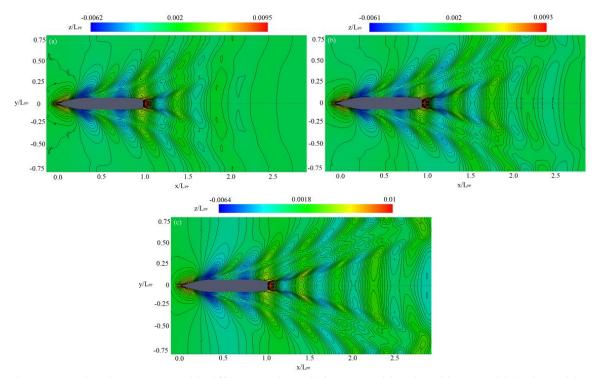
Fig. 7 Wave elevation contours with different mesh resolutions. (a) grid 1; (b) grid 2; (c) grid 3. The position values are normalized using the ship length ( $L_{PP}$ )
