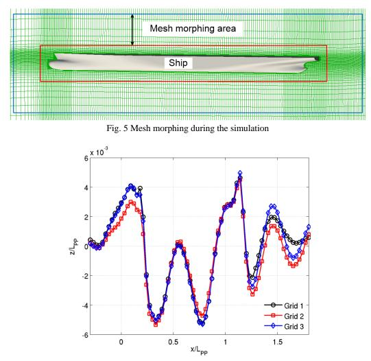
Fig. 6 Wave elevations at the lateral position  $y/L_{PP}=0.0741$  for three different grids (Fr=0.260). The position values are normalized using the ship length ( $L_{PP}$ )
