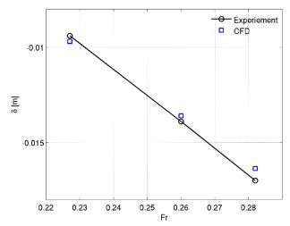
Fig. 16 Sinkage ( $\delta$ ) against Froude number (Fr) in the dynamic case. Experimental data comes from Kim *et al.* (2001)
