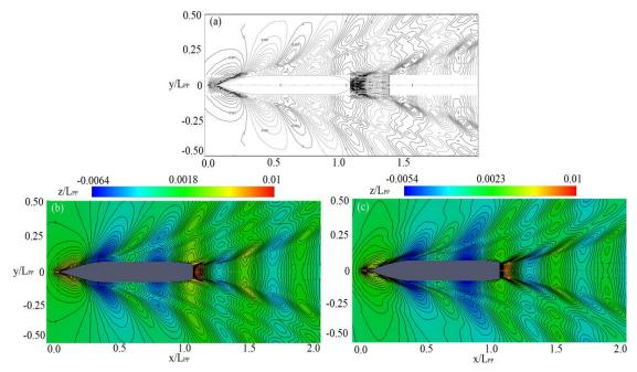
Fig. 8 Comparison of the wave elevation contours between the static and dynamic cases (Fr=0.260). (a) experiment (Hino 2005); (b) static case; (c) dynamic case. The position values are normalized using the ship length ( $L_{PP}$ )
