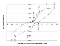
Fig. 2 Lateral load vs. second story displacement-Phase A (Duong 2006)
