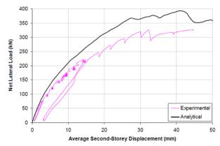
Fig. 5 Phase A Forward Half-Cycle: Lateral Load vs. Second-Storey Displacement (Duong 2006)
