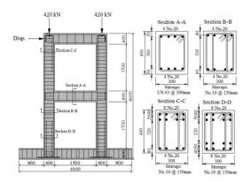
Fig. 1 Frame loads and cross-sections (Güner 2008)
