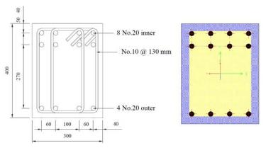
Fig. 9 Section C-C created with Section Designer
