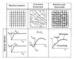
Fig. 4 The modified compression filed theory for membrane elements (Vecchio and Collins 1986)
