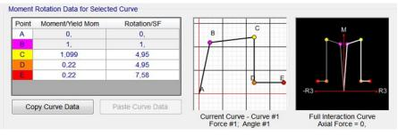
Fig. 8 Moment-rotation curve of P-M3 hinge for Section B-B
