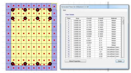
Fig. 11 Section C-C generated fibers
