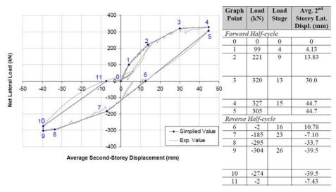
Fig. 3 Simplified diagram and key load stages of test (Duong 2006)
