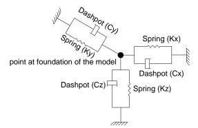
Fig. 4 3D SSI element connected to raft foundation (damper and spring in x, y and z directions)
