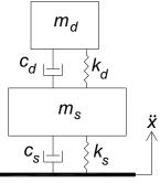
Fig. 5 SDOF system with TMD
