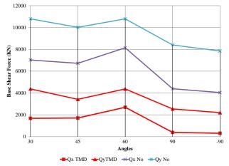
Fig. 12 Base shear in x and y directions of the model with different earthquake exposure angels
