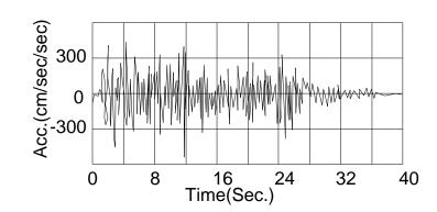
Fig. 2 Accelerograms used for the analyses El Centro
