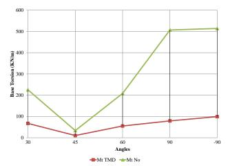
Fig. 13 Base torsion of the model under different earthquake exposure angles
