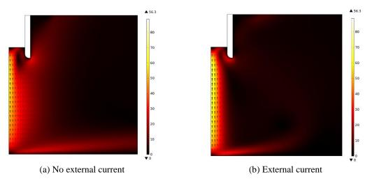
Fig. 12 The velocity fields and equivalence contour (max: 70, min: 10, interval: 12 m/s)
