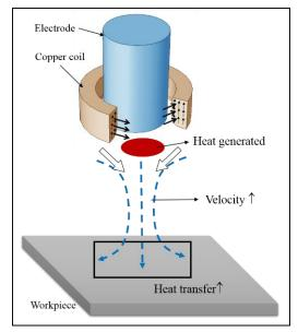
Fig. 8 The diagram of the coil added welding system
