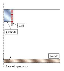
Fig. 9 Computational domain of the coil added system
