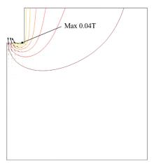
Fig. 3 The azimuthal direction of magnetic flux density (contours, interval: 0.005T) and The current density (arrow line)
