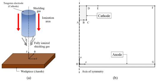
Fig. 1(a) Schematic figure of GTAW, (b) 2D Axi-symmetric model of GTAW
