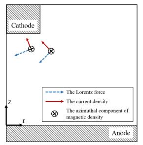
Fig. 6 Schematic figure of interaction between the current density, magnetic density and Lorentz force
