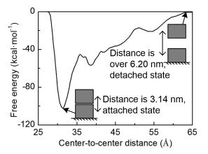
Fig. 3 The plot of the free energy against the center-to-center distance from metadynamics simulation
