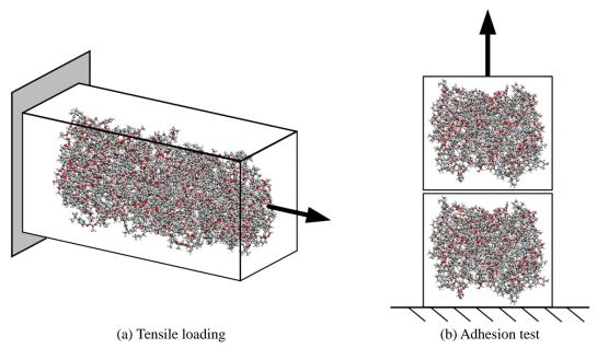
Fig. 1 Mechanical loading cases of the SU-8 to derive parameters for the mesoscopic model
