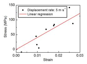
Fig. 2 Stress versus strain data for stretching a SU-8 epoxy chain using the PCFF potential
