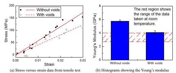
Fig. 5 Tensile test of the mesoscale SU-8 network
