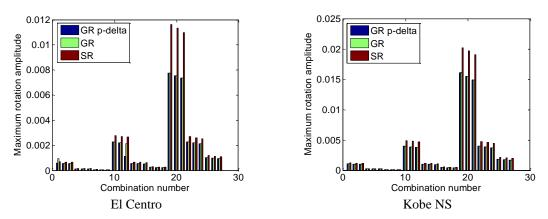
Fig. 7 Variation of maximum rotation as function of the combination number in the case of flexible foundation-mat on Winkler foundation type; (GR p-delta) designates great rotation with p-delta effect; (GR) great rotation without p-delta effect and (SR) small rotation
