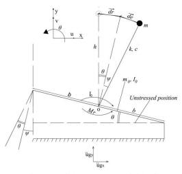
Fig. 4 Flexible structure on rigid soil
