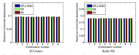
Fig. 10 Variation of maximum horizontal displacement as function of the combination number in the case of flexible foundation-mat on rigid soil; (GR p-delta) designates great rotation with p-delta effect; (GR) great rotation without p-delta effect and (SR) small rotation
