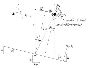
Fig. 2 Free body diagram of the system with uplift showing the considered dependent and independent degrees of freedom
