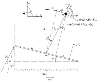
Fig. 5 Free body diagram of the system with uplift showing the considered dependent and independent degrees of freedom
