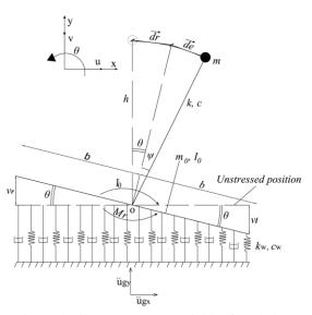
Fig. 1 Flexible structure on Winkler foundation
