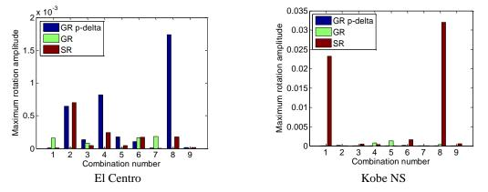
Fig. 9 Variation of maximum rotation as function of the combination number in the case of flexible foundation-mat on rigid soil; (GR p-delta) designates great rotation with p-delta effect; (GR) great rotation without p-delta effect and (SR) small rotation
