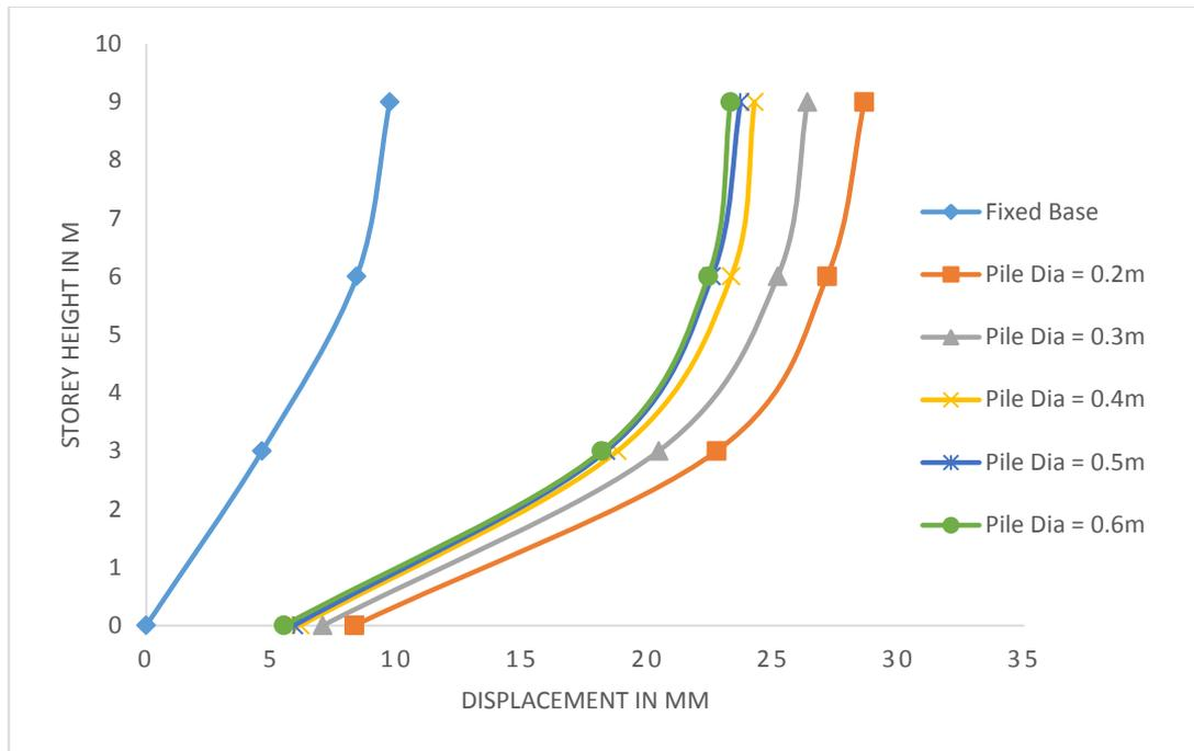
Fig. 6 Effect of pile diameter on displacement
