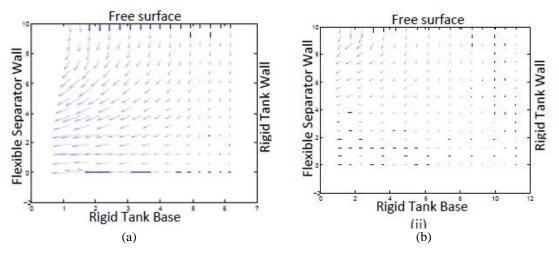
Fig. 13 Velocity vectors at t = 4.20 sec in fluid for (a) L = 5 m and (b) L = 15 m
