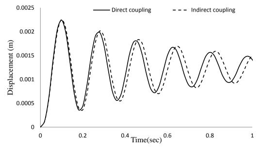
Fig. 4 Tip displacement of the separator wall due to ramp acceleration
