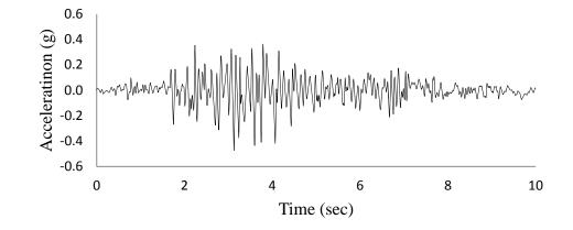
Fig. 6 Horizontal component of Koyna earthquake
