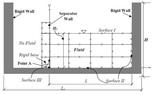
Fig. 1 A typical finite element discretization of tank-water system
