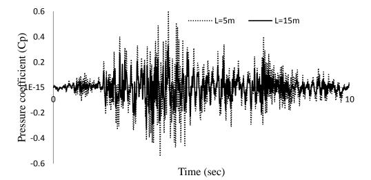
Fig. 9 Hydrodynamic pressure at point A due to Koyna earthquake
