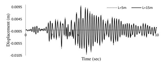
Fig. 7 Tip displacement of separator wall due to Koyna earthquake
