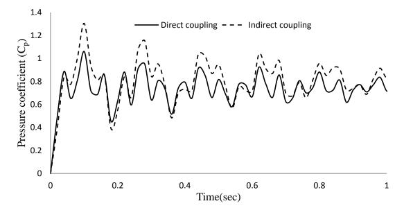
Fig. 5 Hydrodynamic pressure at point A due to ramp acceleration
