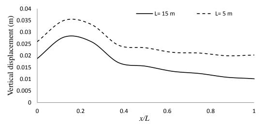
Fig. 12 Sloshed displacement for different length of tank at t = 4.20 sec
