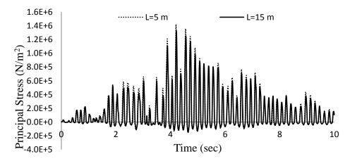
Fig. 8 Major Principal stress at the base of the separator wall due to Koyna earthquake
