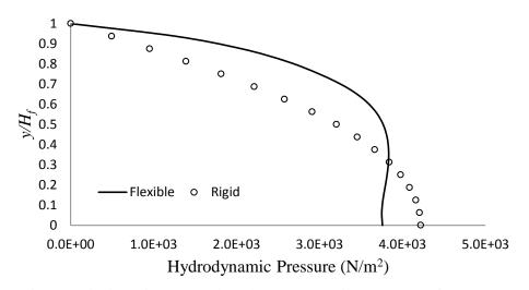
Fig. 10 Hydrodynamic pressure along the separator wall at t = 4.20 sec for L=5 m
