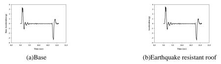
Fig. 27 Input acceleration at base and estimated response at roof of shock 7
