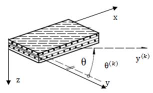
Fig. 1 A laminate with the material and problem coordinate systems
