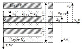
Fig. 2 Coordinate system and layer numbering used for a laminated sheet
