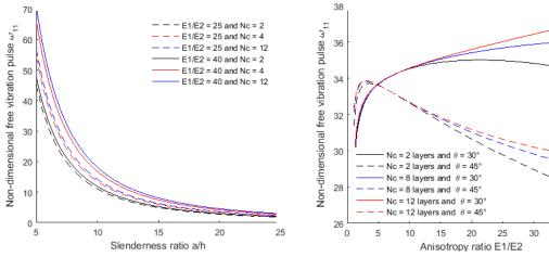
Fig. 6 Variation of the natural frequency  $\omega_{11}$  as a Fig. 7 Variation of the natural frequency  $\omega_{11}$  as a function of the ratio a/h with  $N_c$  and the anisotropy function of the ratio  $E_1/E_2$  with  $N_c$  and the ratio  $E_1/E_2$  as parameters
