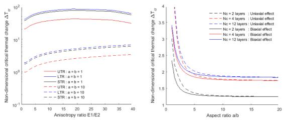
Fig. 4 Variation of the critical temperature  $\Delta T_{cr}$  as a Fig. 5 Variation of the critical temperature  $\Delta T_{cr}$  as a function of the ratio  $E_1/E_2$  with plate size and function of the ratio a/b with  $N_c$  and the direction temperature distribution as parameters
